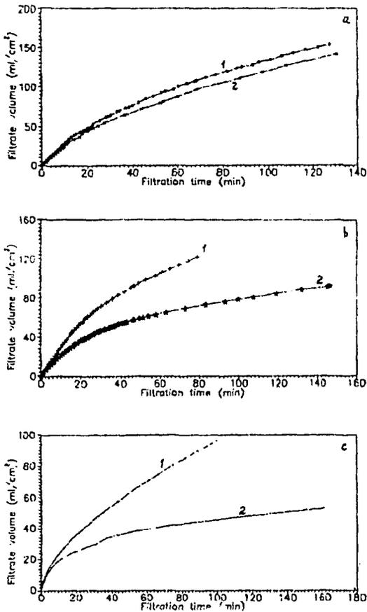
Fig. 3. The filtration throughput of tap water for the membranes with nominal pore sizes of  $0.2 \mu\text{m}$  (a),  $0.4 \mu\text{m}$  (b) and  $1 \mu\text{m}$  (c). The membrane thicknesses are  $20 \mu\text{m}$  (1) and  $10 \mu\text{m}$  (2). The inlet pressure is 0.8 bar
