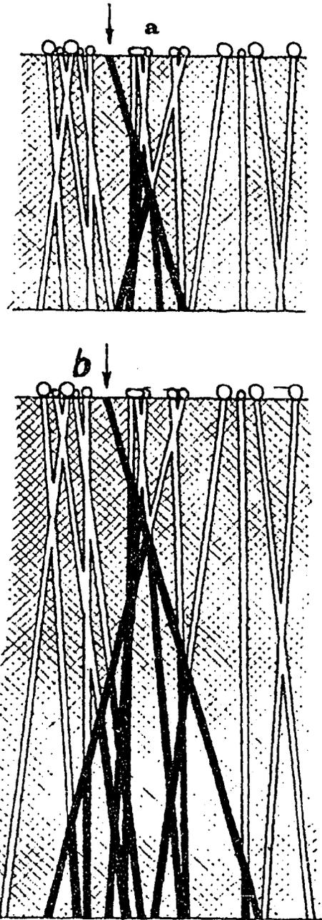
Fig. 4. The cross sections of TM10 and TM20 with the pore diameter of  $0.2 \mu\text{m}$  and pore density of ca.  $3 \times 10^9 \text{ cm}^{-2}$ . All but one of the pores are plugged by particles in the filtration process. The water stream is shown in black. (a) TM10: 21 per cent of the total pore length and 6 pores share in the water flow. (b) TM20: 43 per cent of the total pore length and 12 pores share in the water flow
