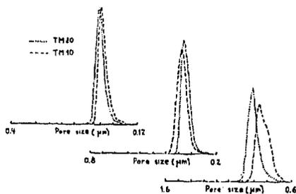
Fig. 1. Differential flow distributions (arbitrary units) as functions of pore diameter for the pairs of track membranes with nominal pore size of 0.2, 0.4 and 1  $\mu\text{m}$  (from left to right)
