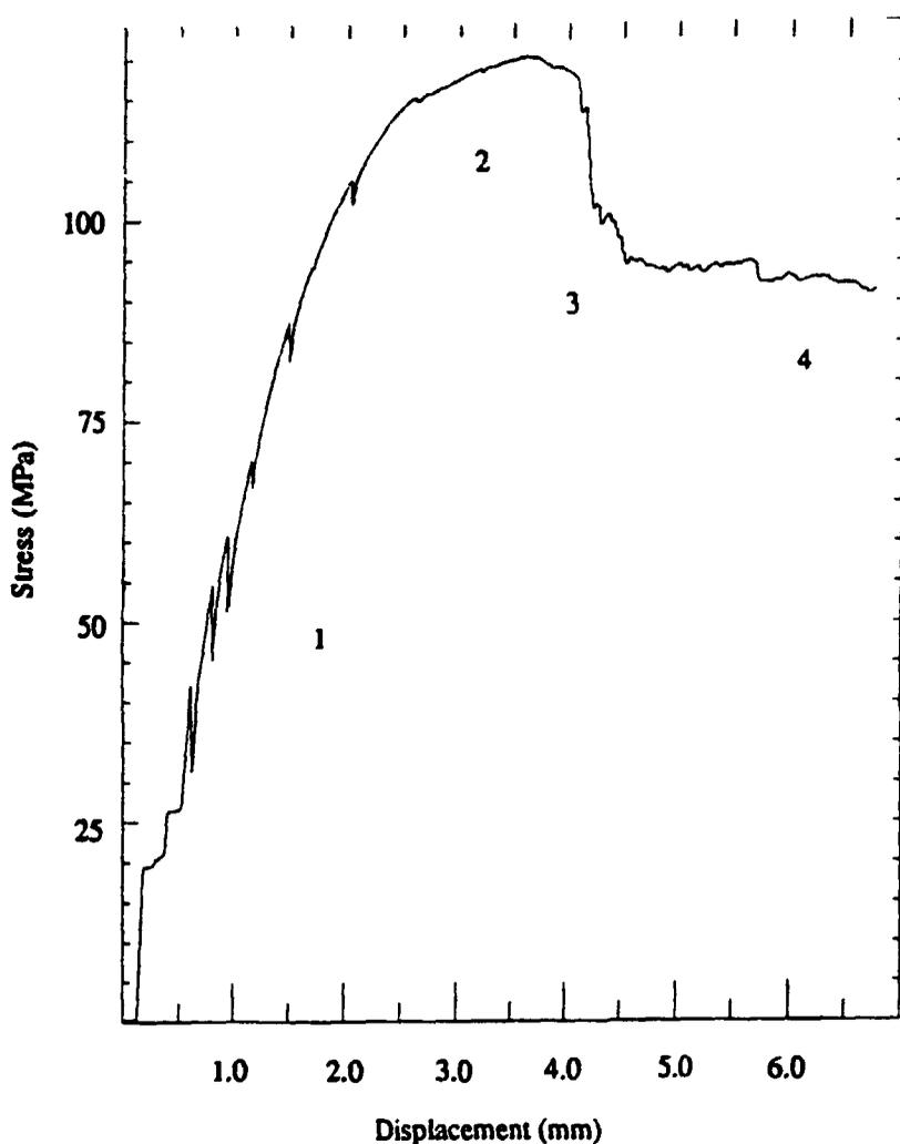
1. Initiation and propagation of cracks within the lower part of the ceramic matrix.
