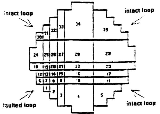
fig. 2 : FLICA-4 radial meshing
