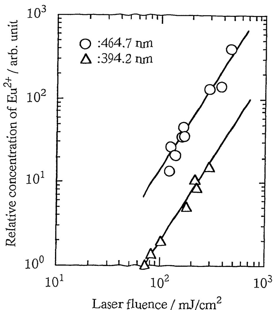
Figure 1. The laser power dependence of the concentration of  $\text{Eu}^{2+}$  vs. the irradiating laser fluence. The slope of the solid lines was 2.0.
