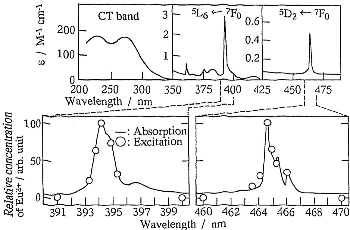
Figure 2. The concentration of  $\text{Eu}^{2+}$  formed by several wavelengths at the irradiating laser fluence of  $290 \text{ mJ/cm}^2$ . The symbols (O) are the normalized concentration of  $\text{Eu}^{2+}$  and the solid lines are the absorption spectra.
