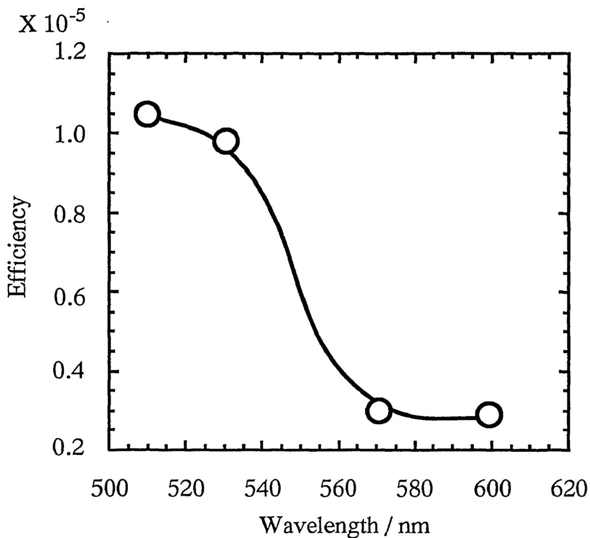
Figure 3 Photoreduction efficiency by the two color and two photon excitation at the same time. The first photon was fixed at the transitions  ${}^5L_6 \leftarrow {}^7F_0$  (394.2 nm) with the fluence of 440 mJ/cm<sup>2</sup>. The efficiency was measured for the second photon at four wavelengths. The photon number second photon was  $9.8 \times 10^{17}$  photon/cm<sup>2</sup> (corresponding to 494 mJ/cm<sup>2</sup> at 394.2nm)
