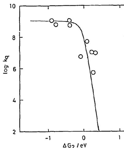
Fig. 2 Plot of  $\log k_q$  vs.  $\Delta G_2$ ;  $k_1 = 1.5 \times 10^9 \text{ mol}^{-1} \text{ dm}^3 \text{ s}^{-1}$ ,  $k_{-1}/Z = 0.25$  and  $\Delta G_2^*(0) = 10.1 \text{ kJ mol}^{-1}$ .
