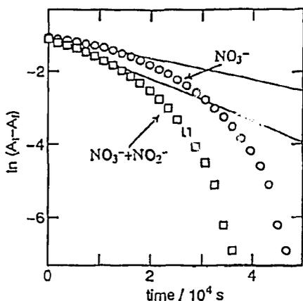
Fig. 6 Pseudo first order plot for the oxidation of U(IV) by  $\text{NO}_3^-$  in dark (O) and the same plot for the solution, in which  $\text{HNO}_2$  (0.03M) was previously added, (□) under the condition:  $[\text{U(IV)}] = 0.009 \text{ M}$ ,  $[\text{NaNO}_3] = 0.3 \text{ M}$ , and  $[\text{H}^+] = 0.5 \text{ M}$  at at ionic strength = 3.5 M and at 40 °C.
