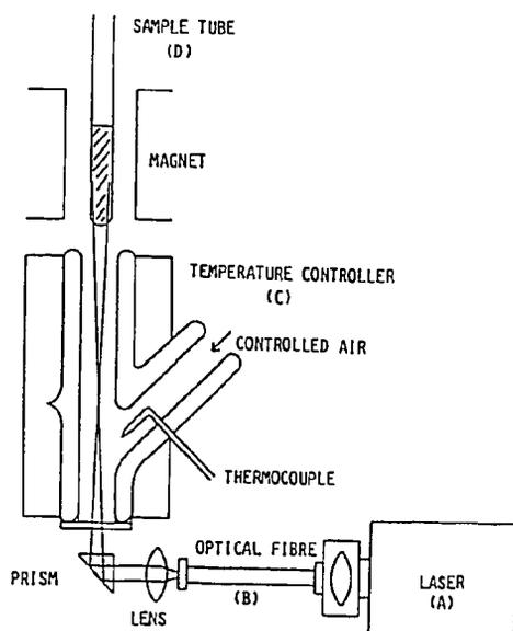
Fig. 3 Scheme of laser-irradiation system. The system consists of four main components: (A) laser, (B) optical fibre, (C) temperature controller and (D) sample tube.
