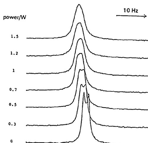
Fig. 4  $^{17}\text{O}$  NMR spectra of uranyl oxygens as a function of laser power (W).
