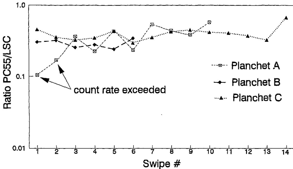
Figure 2: Comparison of the activity measured on Ontario Hydro swipe media using the PC-55 and swipe/LSC
