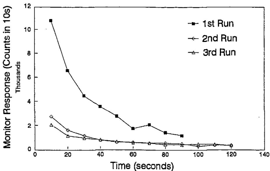
Figure 4: Time required for the Whitlock VSC 5000 surface contamination monitor to stabilize after being turned on
