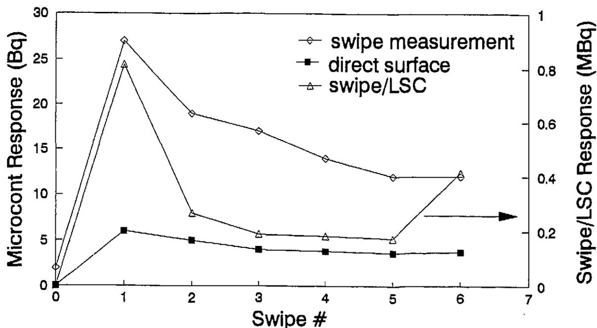
Figure 7: Comparison on Herfurth Microcont Monitor with LSC measurements (direct and indirect)
