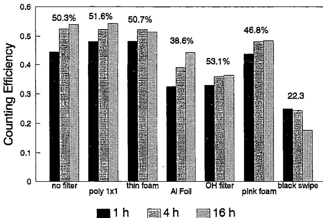
Figure 1: Counting efficiencies of various swipe media in Ultima Gold liquid scintillation cocktail
