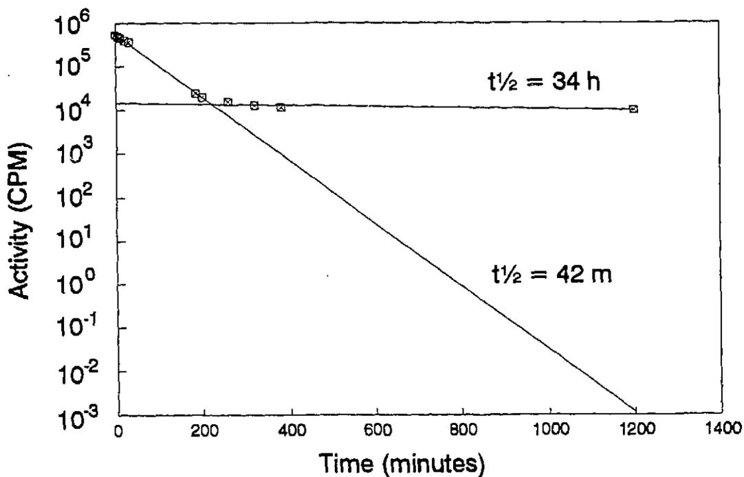
Figure 3: Activity loss, over time, from an Ontario Hydro swipe media measured with the PC-55 proportional counter
