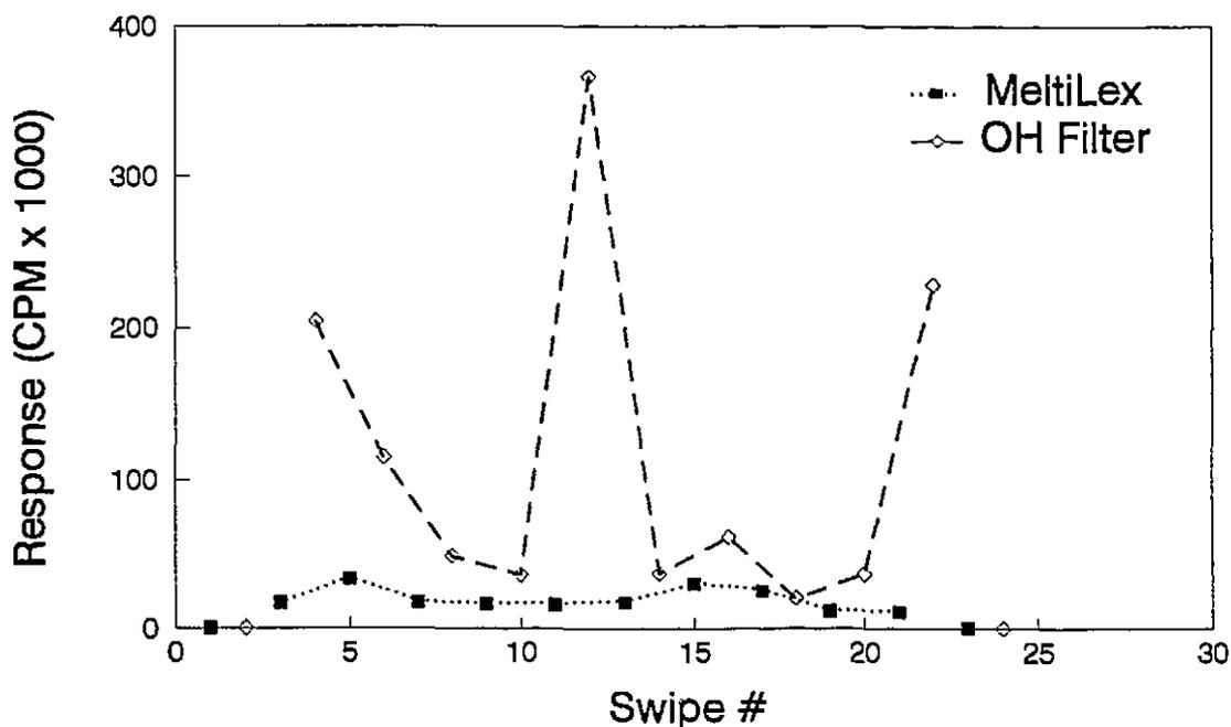
Figure 6: Response of MeltiLex scintillant as a swipe media compared to the activity measured with an Ontario Hydro swipe in Ultima Gold liquid scintillation cocktail. The same surface was alternately swiped with each media. Swipes #1, 2, 23 and 24 are background samples.
