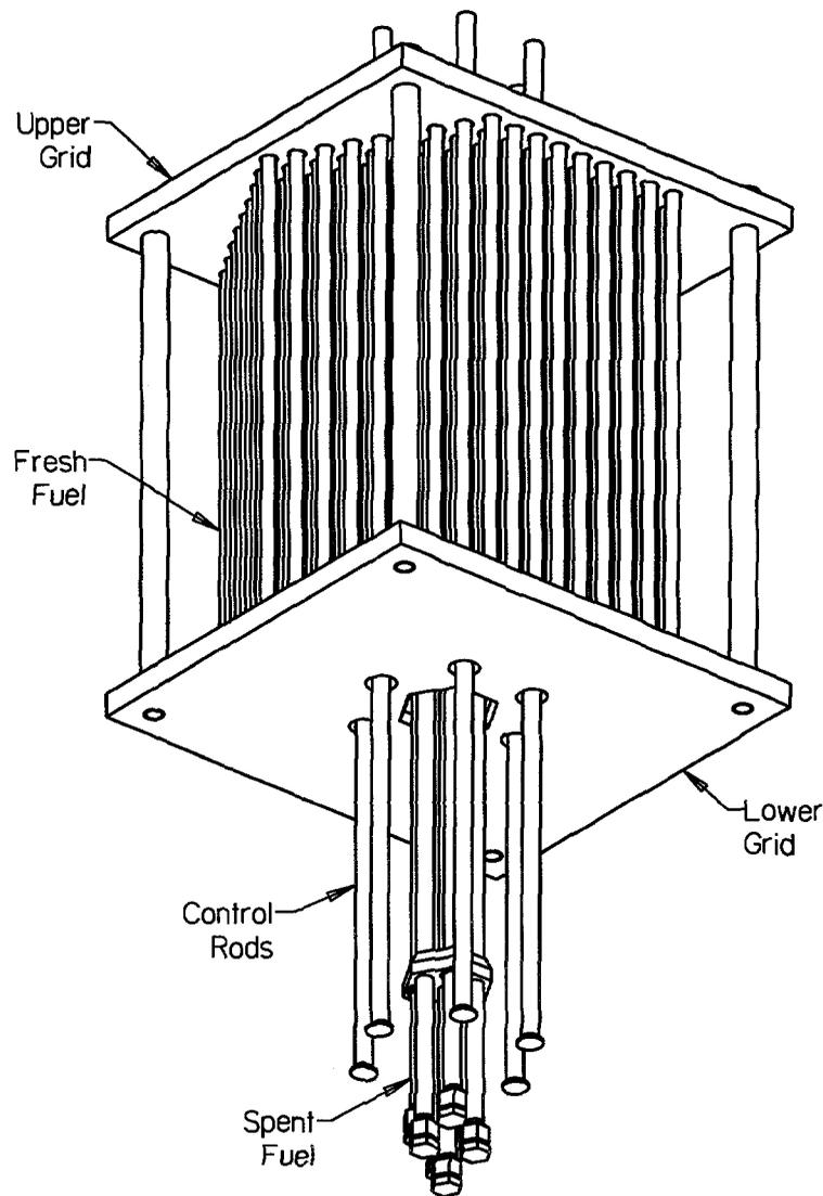
**Figure 3.** View of the SFSX critical assembly from below showing the spent fuel bundle.
