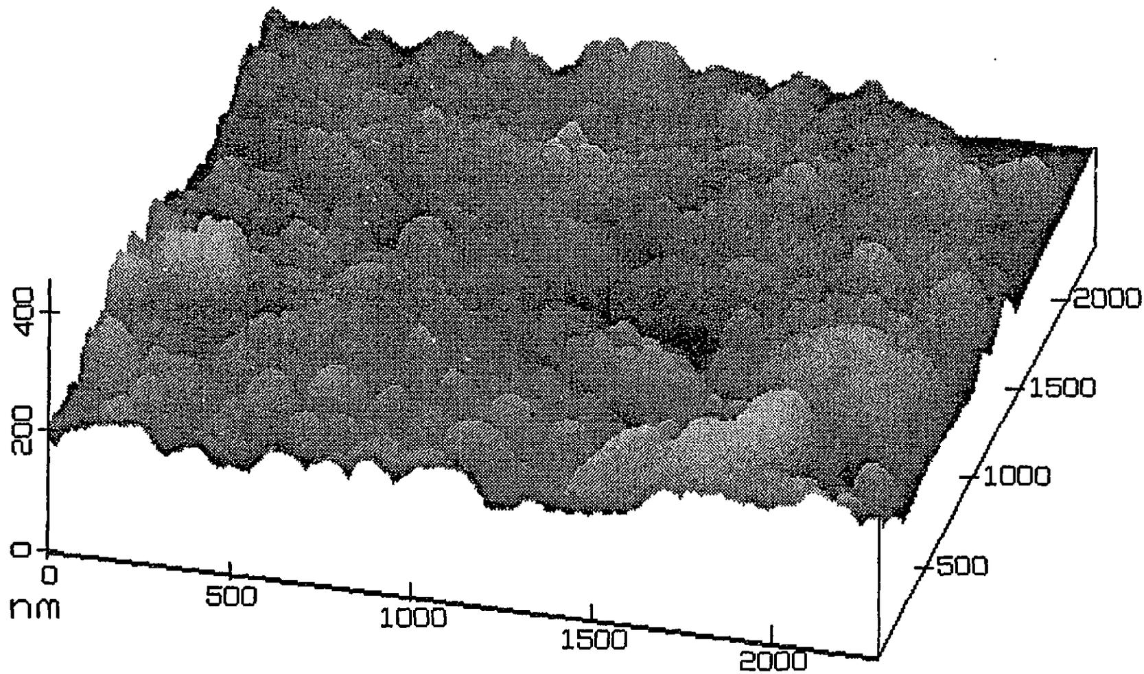
Fig. 14. A 5000 nm × 5000 nm three-dimensional view illustrating one of the crystalline regions.
