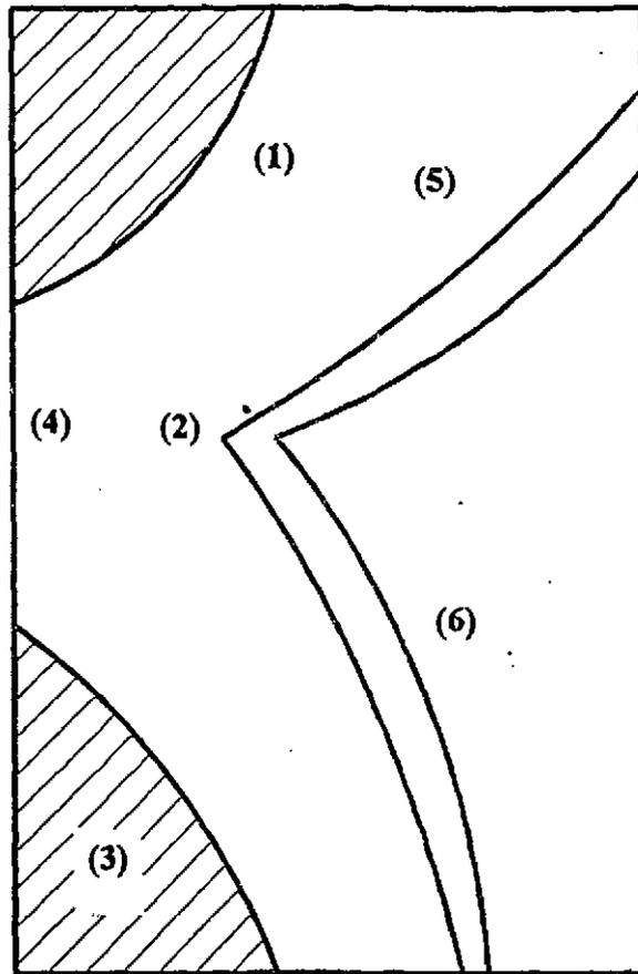
**Fig. 10.** Map of the locations on the Zr-2.5Nb specimen where the Raman spectra were obtained. The lines indicate approximate locations of distinct changes in the coloration of the surface film. The cross-hatched areas were much darker in color than the rest of the sample.
