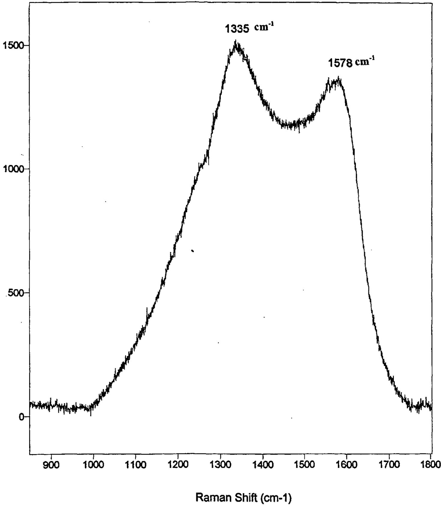
**Fig. 11.** The Raman spectrum at location 5 (in Fig. 10) on an expanded vertical scale. Note the peak at 1335 cm<sup>-1</sup>.
