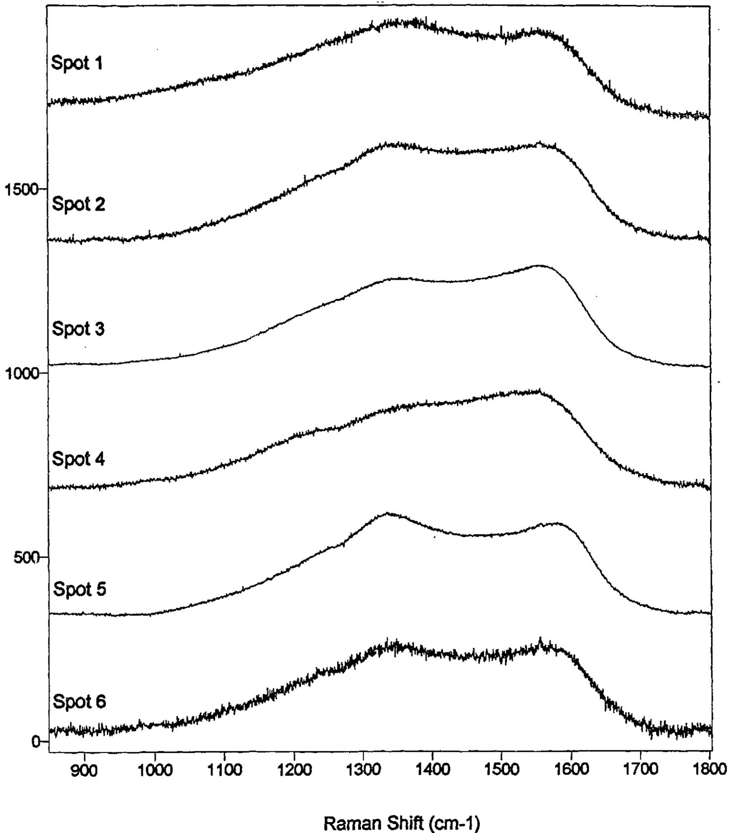
Fig. 9. First-order Raman spectra of laser-generated thin film on Zr-2.5Nb substrate at locations indicated on Fig. 10. Note the broad triangular structure peaking at  $1560\text{ cm}^{-1}$ , with a base stretching from  $1000$  to  $1600\text{ cm}^{-1}$ .
