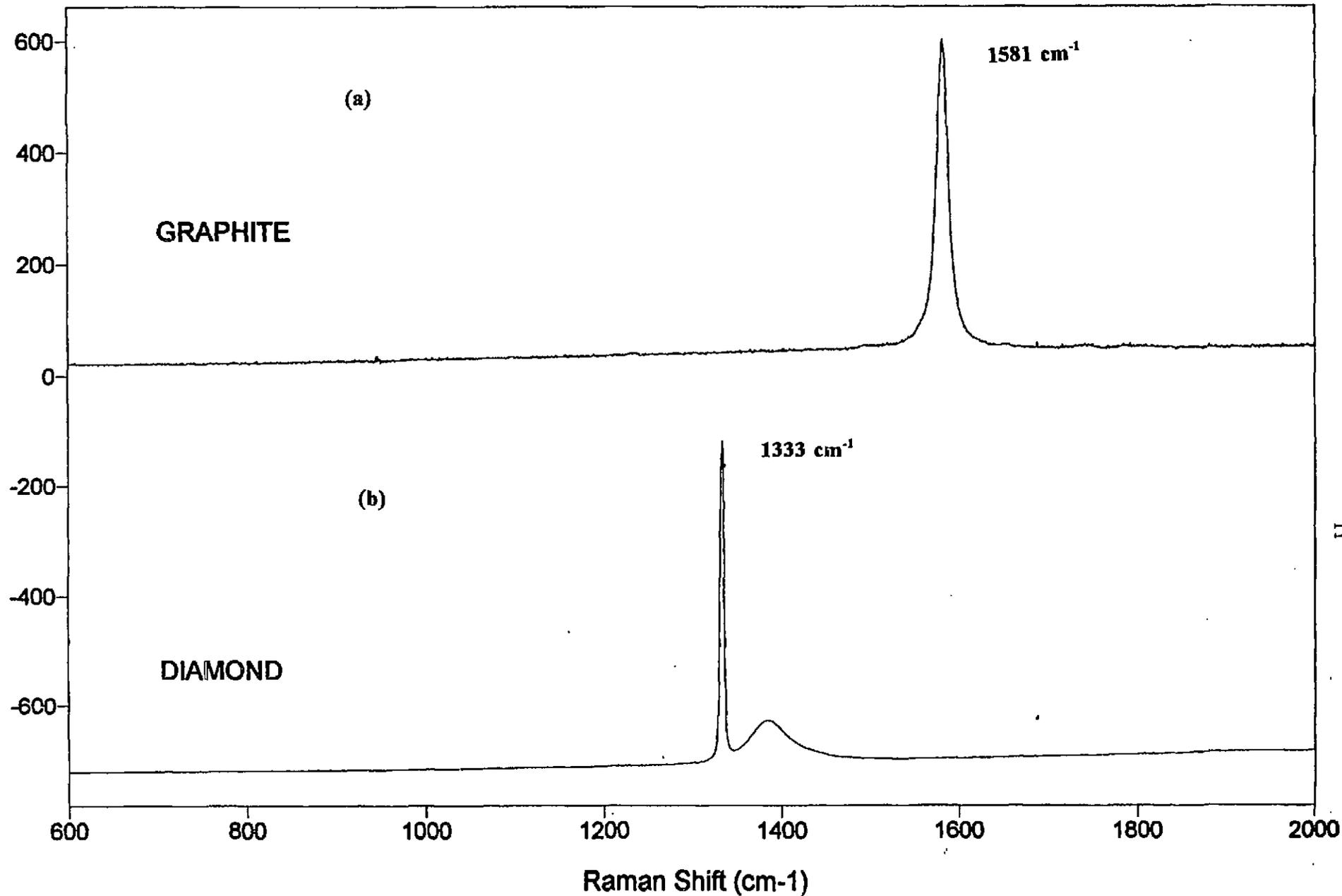
Fig. 5. (a) First-order Raman spectrum of highly-ordered pyrolytic graphite (HOPG). The peak is at 1581 cm<sup>-1</sup>. (b) First-order Raman spectrum of industrial diamond. The peak is at 1333 cm<sup>-1</sup>. The feature at the longer wavenumbers is probably from impurities.
