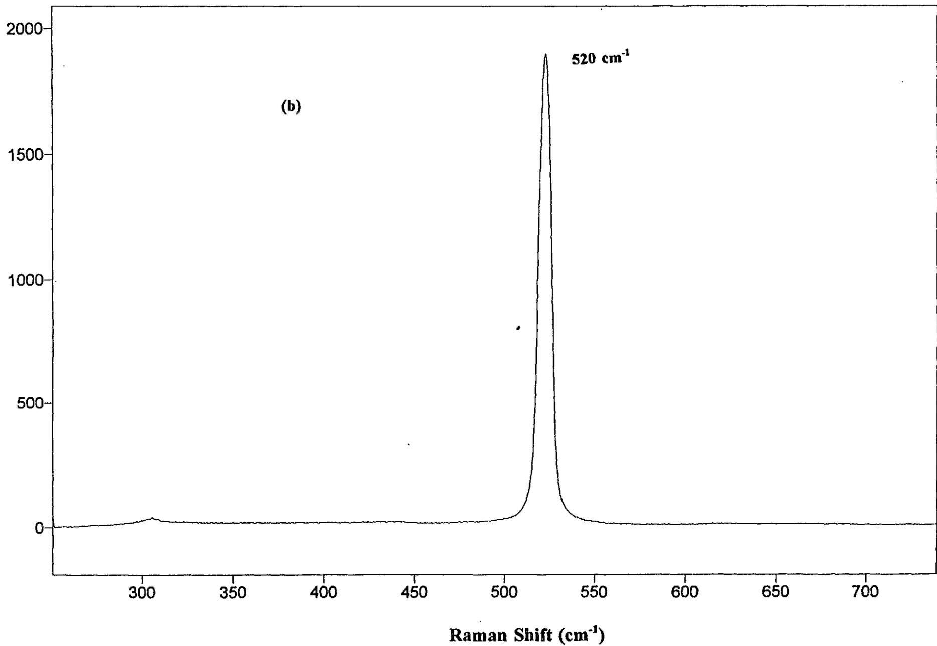
Fig. 8. (b) The silicon line at 520 cm<sup>-1</sup> from the silicon substrate.
