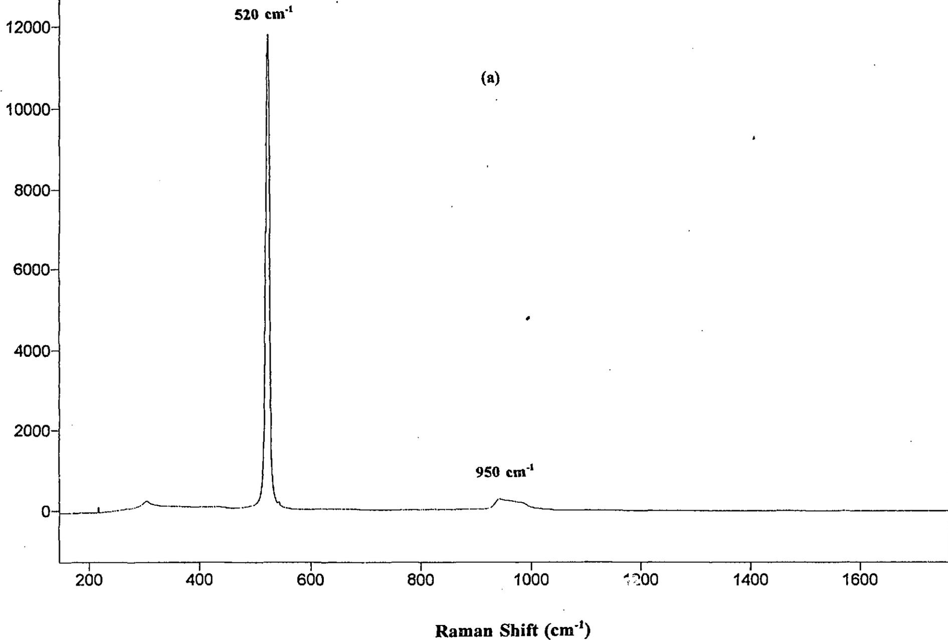
Fig. 7. (a) First-order Raman spectrum of Si(110) substrate with the silicon line at 520 cm<sup>-1</sup>. The smaller feature at 950 cm<sup>-1</sup> (expanded in Fig. 7b) is probably from silicon oxide on the surface.
