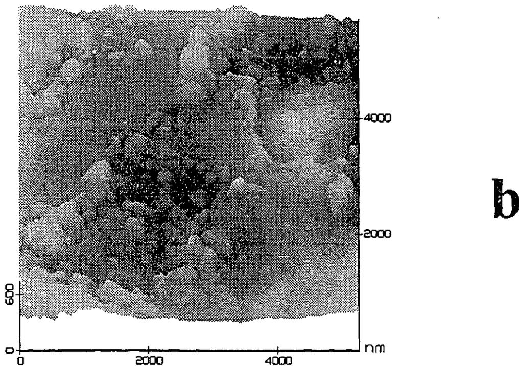
**Fig. 12.** (a) An  $18\ \mu\text{m} \times 18\ \mu\text{m}$  topview AFM image acquired in the darker-colored region of the sample. (b) A  $5000\ \text{nm} \times 5000\ \text{nm}$  three-dimensional view illustrating one of the crystalline regions.
