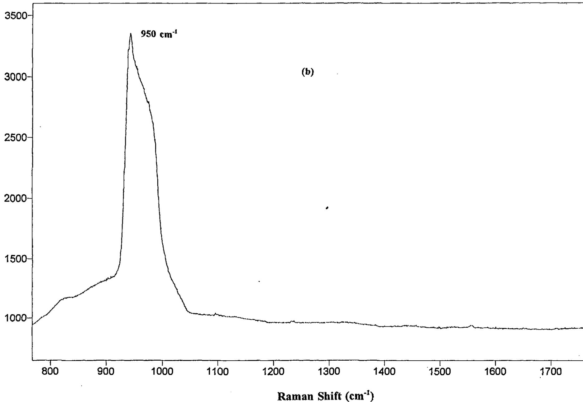
**Fig. 7. (b)** The 800 -1800 cm<sup>-1</sup> region of the Raman spectrum of Si<110> from Fig. 7(a) is replotted with an expanded vertical scale. The feature at 950 cm<sup>-1</sup> is probably from silicon oxide. No features are seen in the spectrum above ~1050 cm<sup>-1</sup>.
