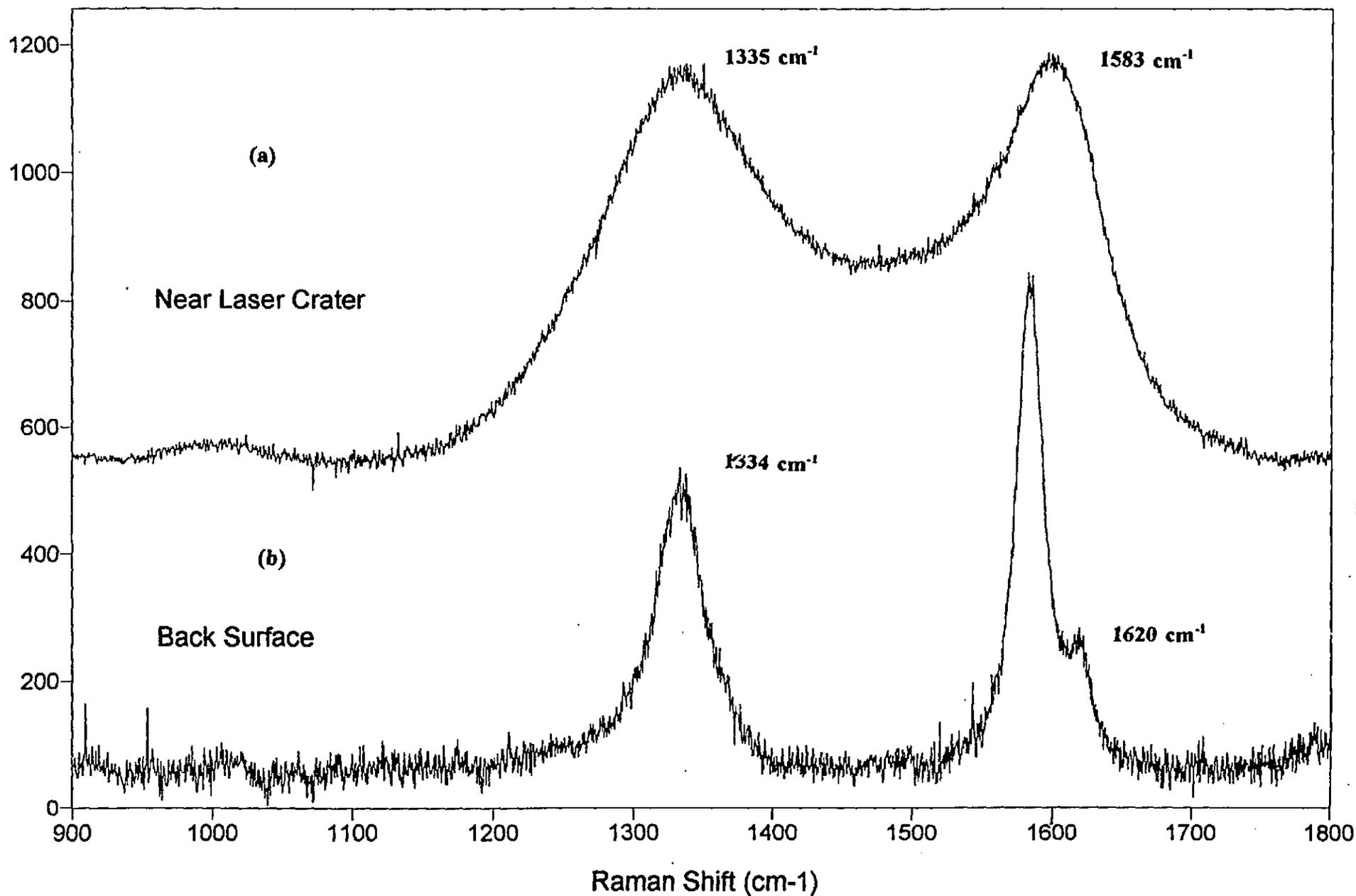
Fig. 6. (a) First-order Raman spectrum of POCO graphite on the back surface (unirradiated surface). The peak at  $1583\text{ cm}^{-1}$  is due to the in-plane vibrations of the layers. The second peak at  $1335\text{ cm}^{-1}$  is ascribed to structural imperfections associated with in-plane vibrations. (b) First-order Raman spectrum of laser-irradiated POCO graphite near a laser crater. Note the broadening of the lines and a small frequency shift as well.
