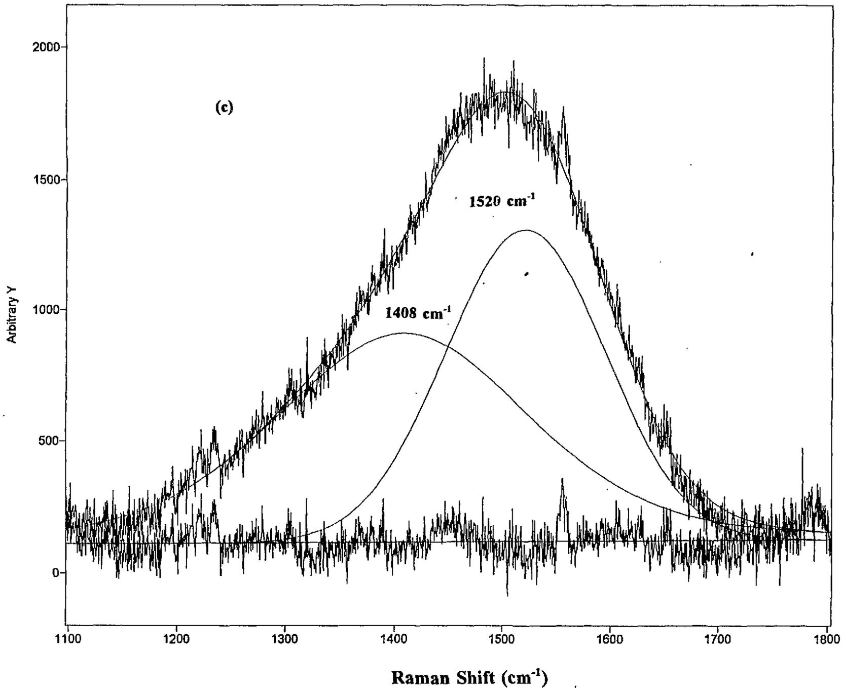
Fig. 8. (c) Line fit to the Raman profile from Fig. 8a, with two peaks at 1408  $\text{cm}^{-1}$  and 1520  $\text{cm}^{-1}$ .
