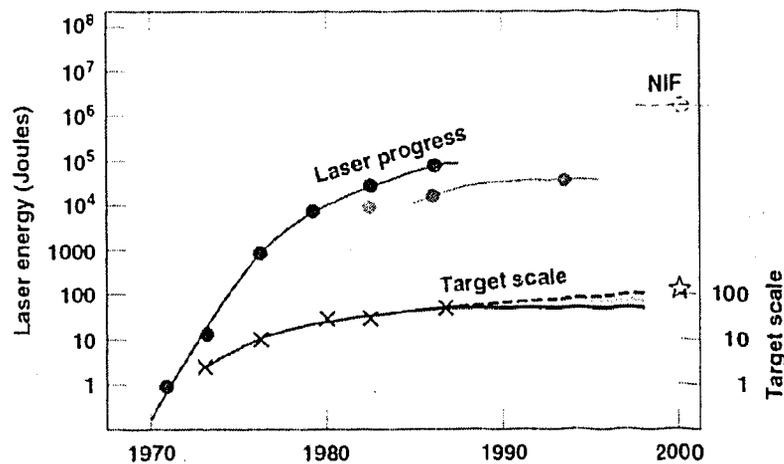
Figure 2: The laser energy (left vertical scale) used to irradiate increasingly large fusion targets is shown as a function of a 30 year development cycle. The associated increase in target scale is shown on the right vertical axis. The dotted line on the curve between now and the year 2000 shows that full scale experiments of target physics issues are being conducted using the Nova laser, but an integrated target demonstration will require a laser delivering energy exceeding 1 megajoule.
