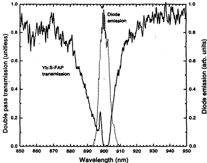
Figure 17. Yb:S-FAP absorption spectra for a double-passed rod with  $1.26 \times 10^{19}$  Yb/cm<sup>3</sup> and an experimental InGaAs diode array emission spectra taken at 2.1 kW peak power output and a 1 ms pulse length with an input cooling water temperature of 10.6 °C
