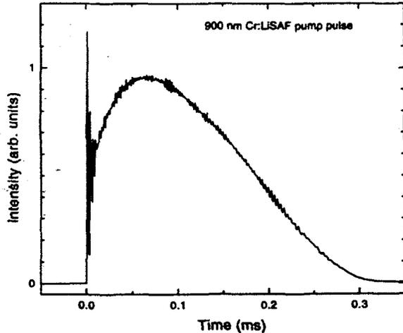
Figure 3. Temporal output pulse shape from the free running Cr:LiSAF oscillator that was used as a surrogate pump source for the laser diode array.
