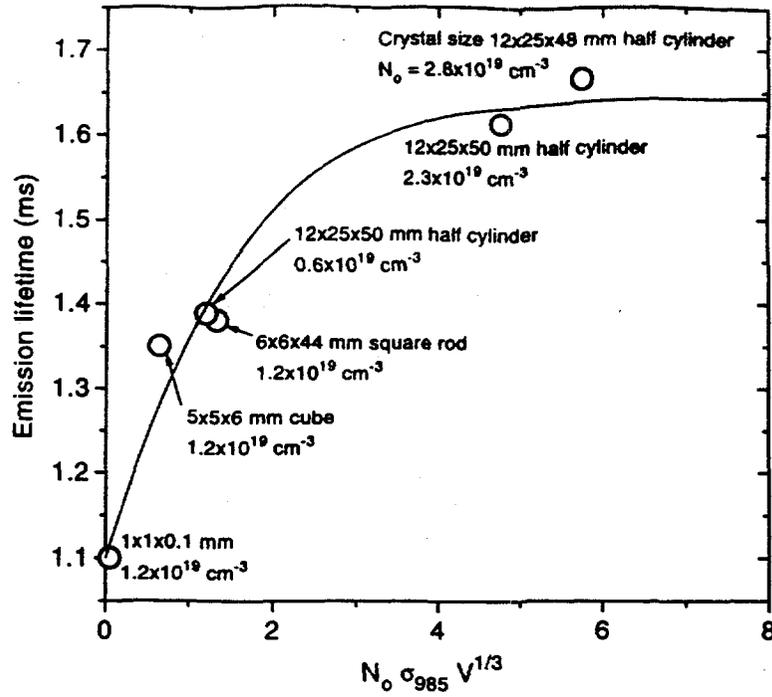
Figure 13. Yb:S-FAP emission lifetime versus the product of the Yb<sup>3+</sup> number density  $N_0$ , polarization averaged 985-nm absorption cross section  $\sigma_{985}$ , and cube root of the crystal volume  $V$ , for six different crystal shapes and Yb<sup>3+</sup> concentrations. The solid line is a fit to the data using a radiation trapping model.
