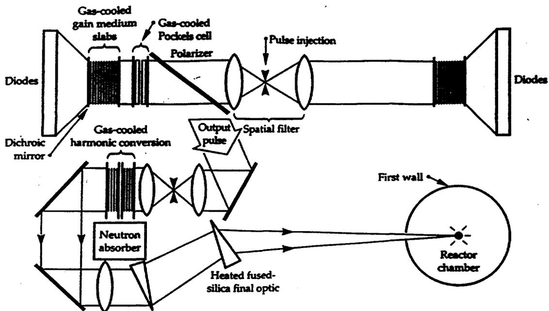
Figure 1. Component sketch of a single beamline from a conceptual diode-pumped solid-state laser based driver for an inertial fusion energy power plant recently developed by Orth and co-workers.<sup>6</sup>
