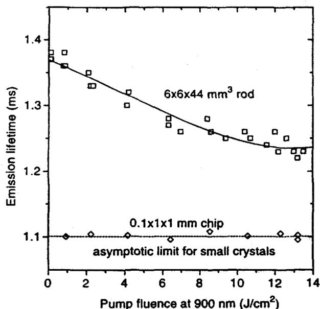
Figure 14. Yb:S-FAP emission lifetime of a 6x6x44 rod (squares) and a  $\sim 0.1 \text{ mm}$  thick chip (diamonds) as a function of pump fluence. The rod experiences a reduction in radiation-trapped lifetime effects due to bleaching at the larger fluences, while the chip shows no signs of radiation trapped effects.
