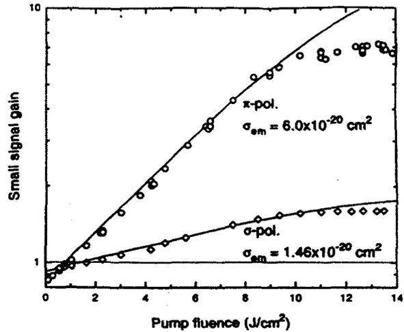
Figure 11. Small signal gain of Yb:S-FAP rod, with either  $\sigma$  or  $\pi$  polarized at 1047 nm light as noted, is shown with the same pumping conditions used for Figs. 5, 7, and 9. The emission cross sections obtained from a numerical fit to the data below 10 J/cm<sup>2</sup> are shown as solid lines.
