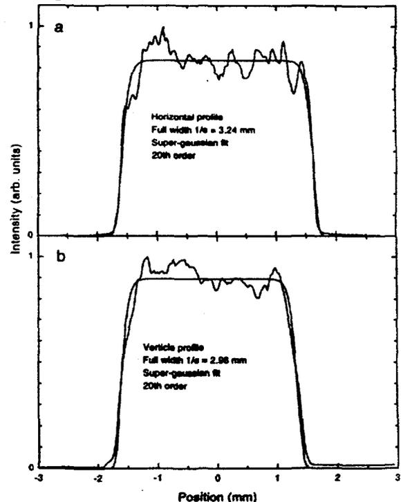
Figure 4. Spatial profile of Cr:LiSAF oscillator 1.2 J pulse at the input of the sample test region.
