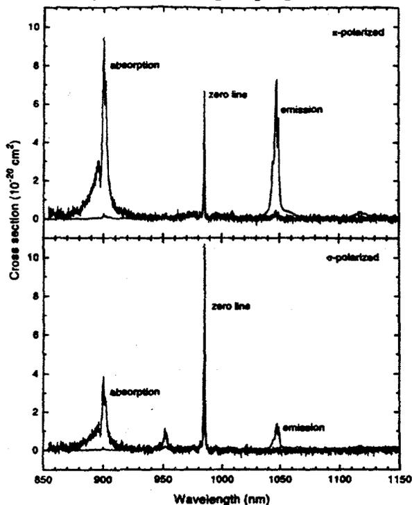
Figure 2. Absorption and emission spectra of Yb<sup>3+</sup> doped Sr<sub>5</sub>(PO<sub>4</sub>)<sub>3</sub>F (S-FAP) for both  $\pi$  and  $\sigma$ -polarizations along with a corresponding energy level diagram.<sup>3</sup> Note that the primary absorption and emission peaks are predominantly  $\pi$ -polarized (parallel to the optical axis).
