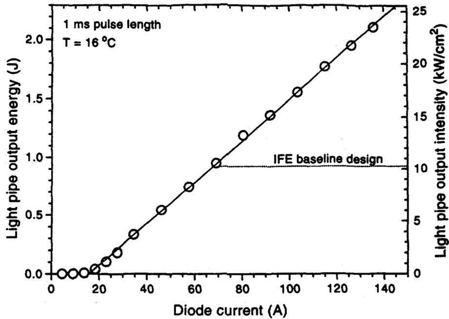
Figure 16. InGaAs diode array energy and intensity verses diode drive current after concentration in a light pipe assembly. The baseline diode intensity in the IFE power plant conceptual design<sup>6,7</sup> of 10.2 kW/cm<sup>2</sup> is noted for comparison.
