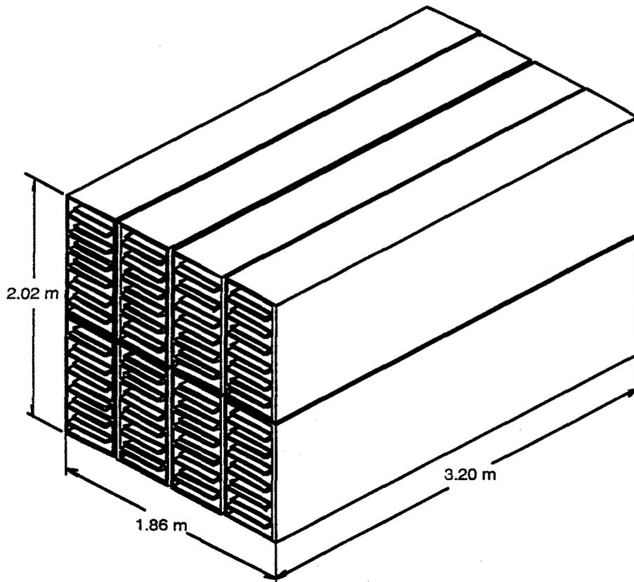
**FIGURE 3.** Folded waveguide array for ITER
