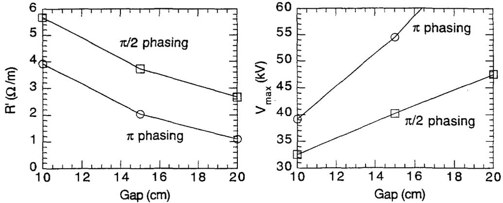
**FIGURE 2.** Loading resistance vs. separatrix-first wall gap (left), and maximum rf voltage vs. gap (right) for phasings of  $\pi$  and  $\pi/2$  between adjacent current straps.
