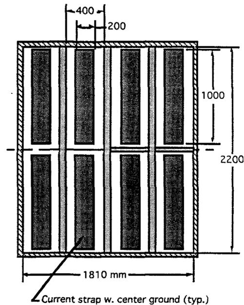
FIGURE 1. View from the plasma of the ITER in-port antenna.
