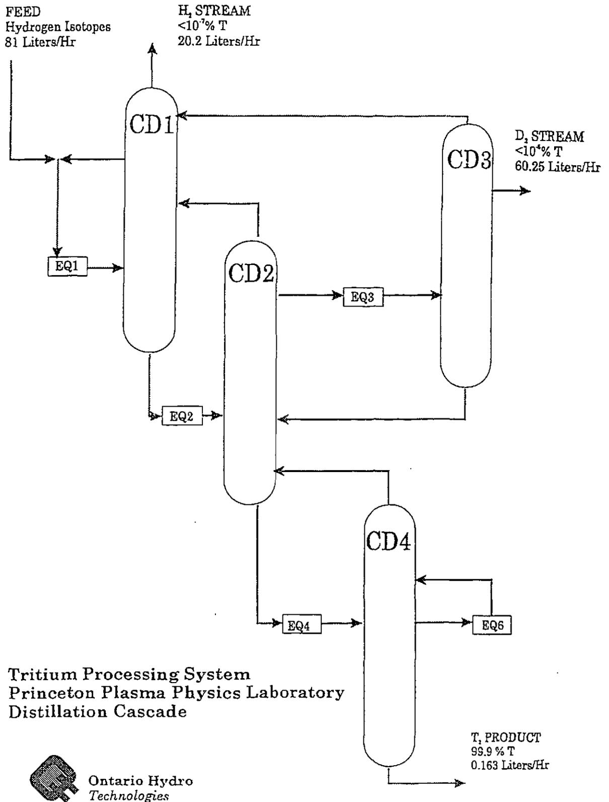
Figure 9. Flow schematic of PPPL TPS cryogenic distillation system.
