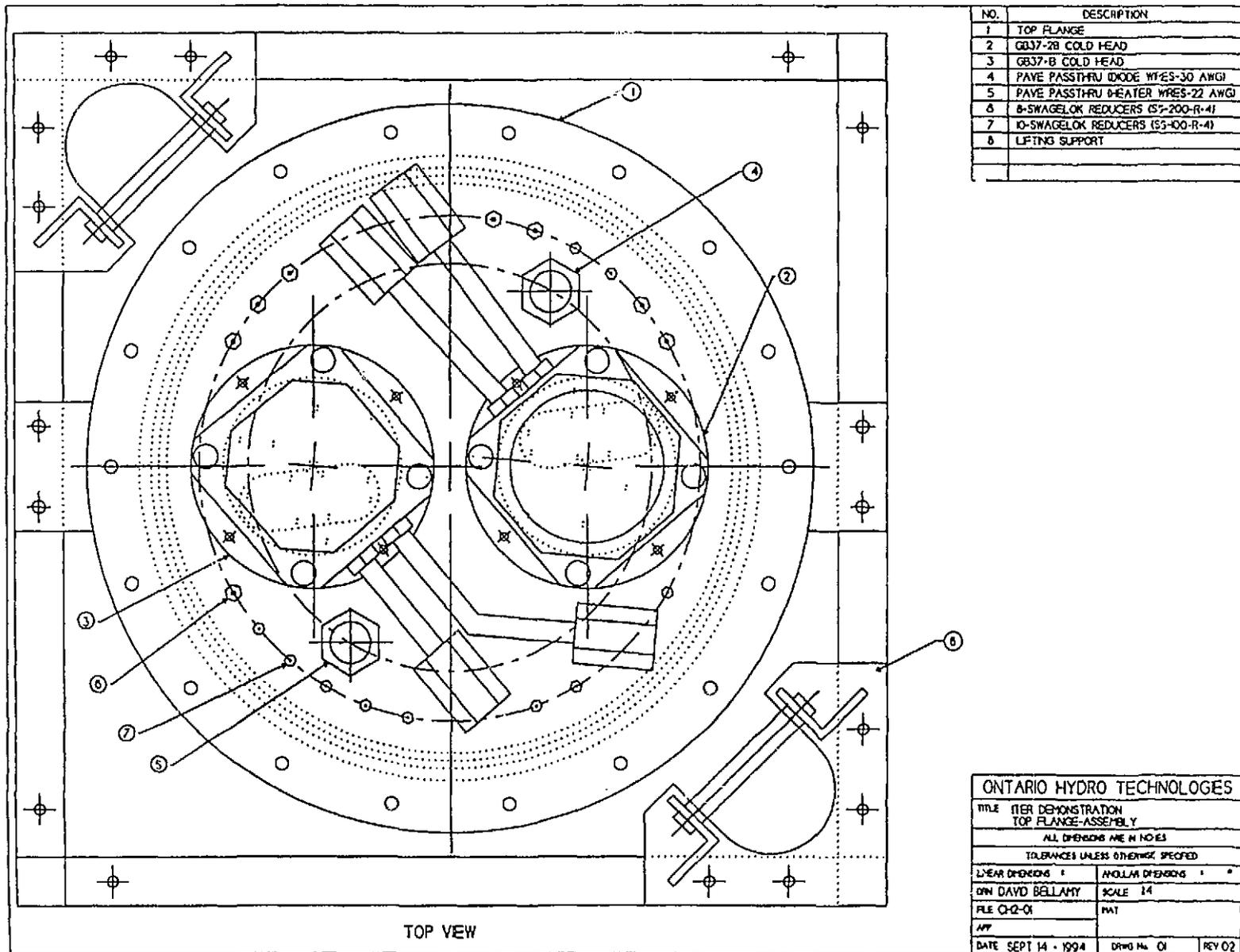
Figure 3. Drawing of the cold box flange.
