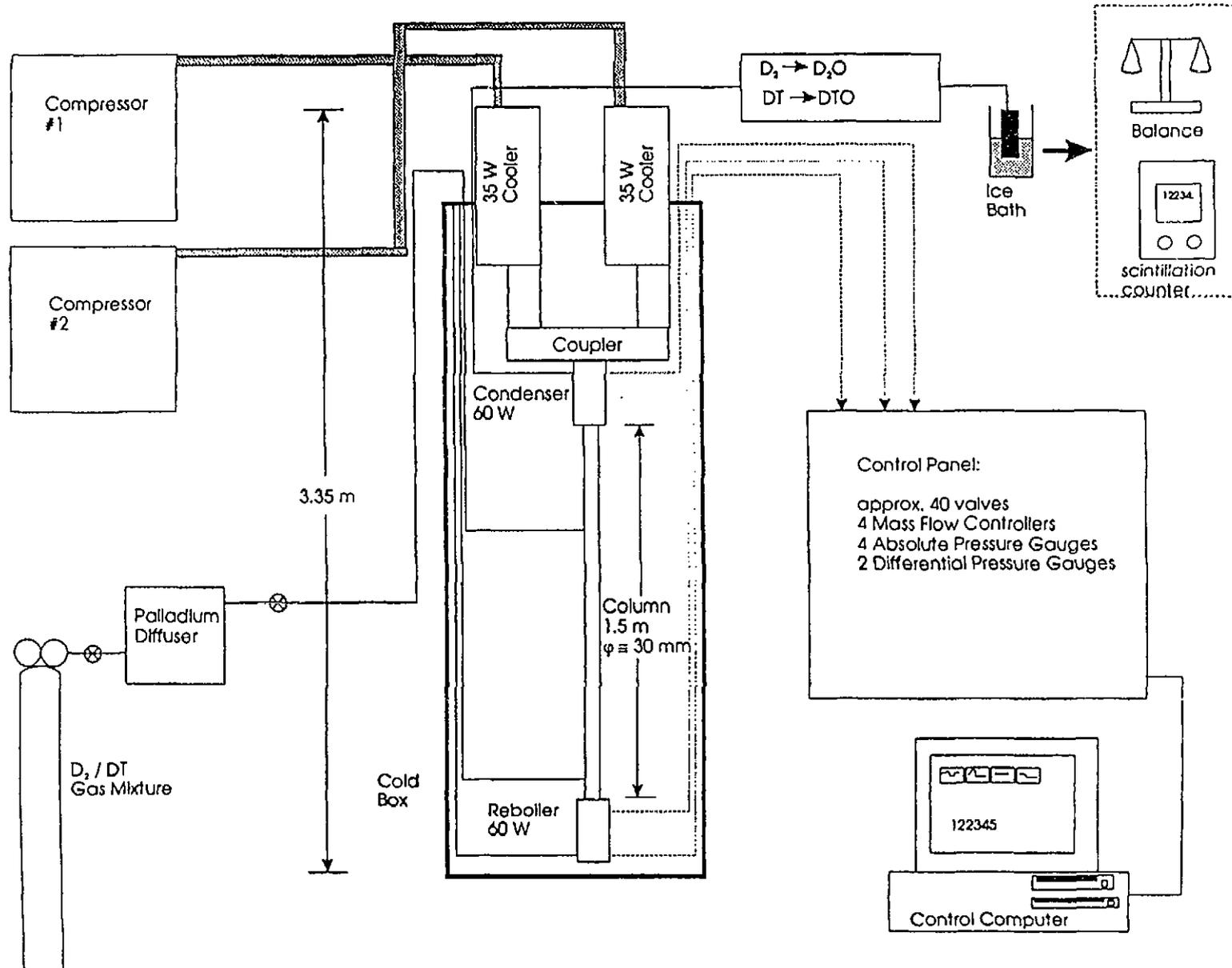
Figure 1. Schematic diagram of Low-inventory Cryogenic Distillation test facility at Ontario Hydro Technologies.
