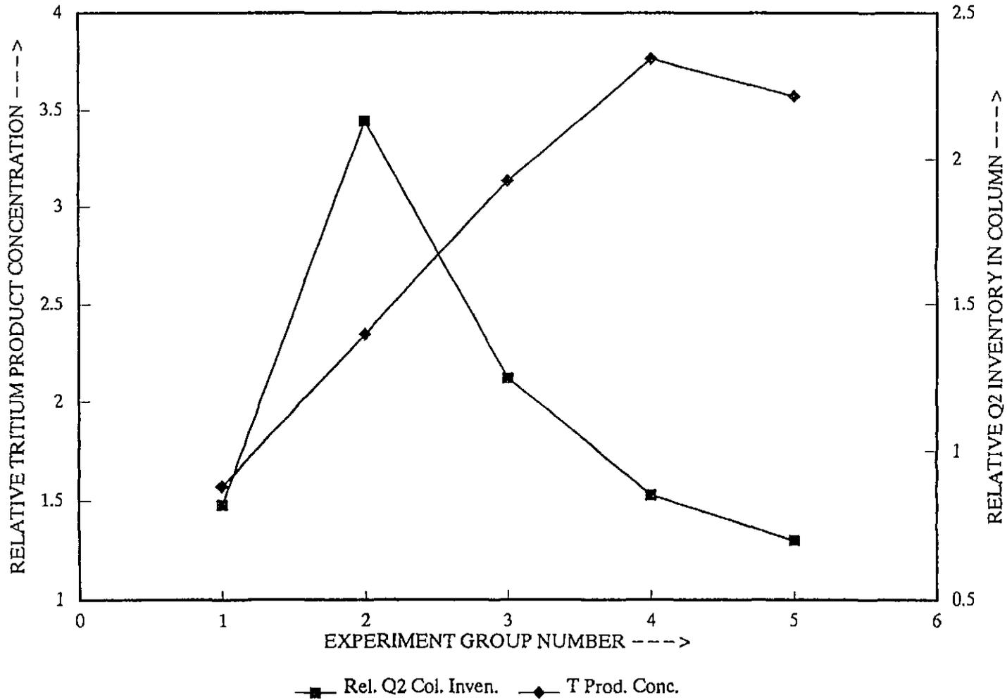
Figure 7. Effect of start-up procedure on tritium separation performance (results from 4.6-mm column tests).
