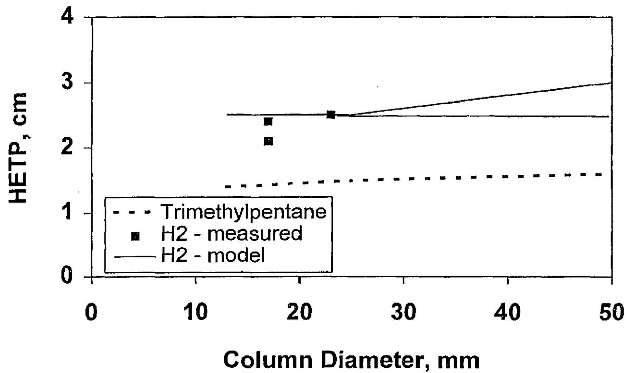
Figure 5. Summary of HETP versus column diameter estimates for Heli-Pak B.
