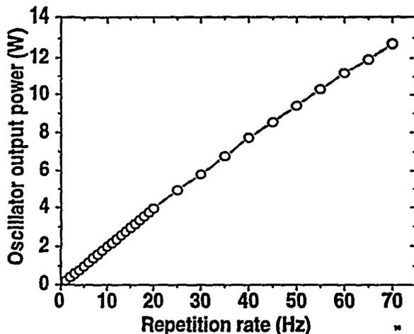
Figure 8. Diode-pumped copper block heat sinked Yb:S-FAP rod-oscillator operating at up to 70 Hz. A 500  $\mu s$  pulse with 120A of drive current were utilized.
