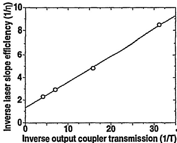
Figure 7. Diode-pumped Yb:S-FAP inverse laser slope efficiency versus inverse output coupler transmission for a diode-pumped free-running oscillator cavity. The Y-intercept and slope provide a measure of the intrinsic laser slope efficiency and the cavity losses, respectively.
