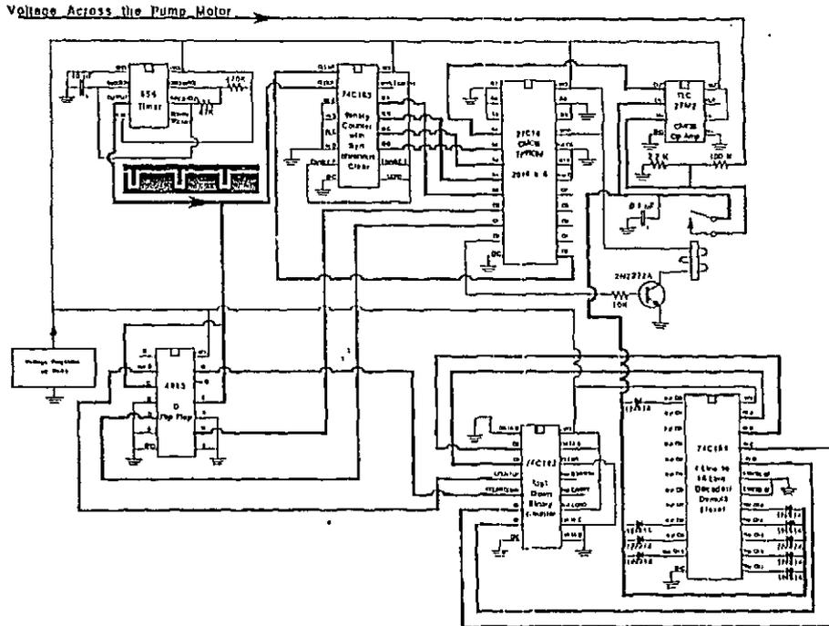
Fig. 11 Circuit diagram of a conditioner for solar powered water pumping system.
