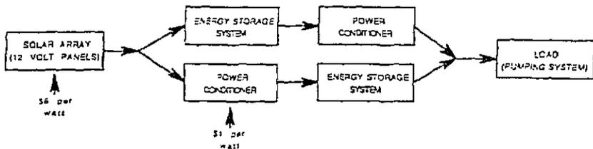
Fig. 8 Shows a block diagram of typical type of small-scale solar powered water pumping system.
