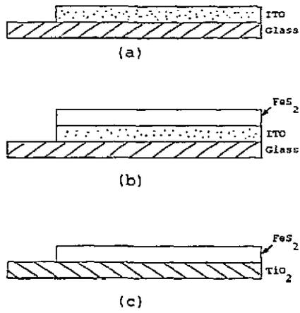
Fig. 7 Show the schematic structure of photoanode.
