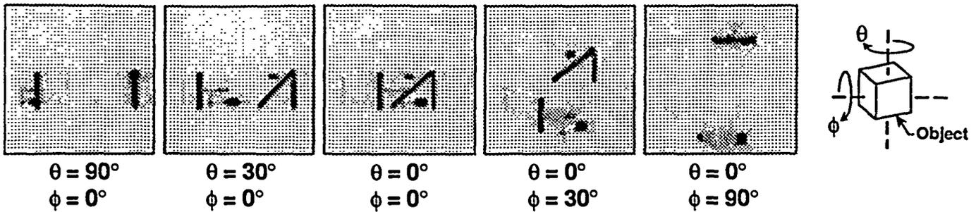
Fig. 3. Views of the 3-D reconstruction of the test object at various orientations. Each image in the figure is a rendered perspective, not a simple projection, of the object.
