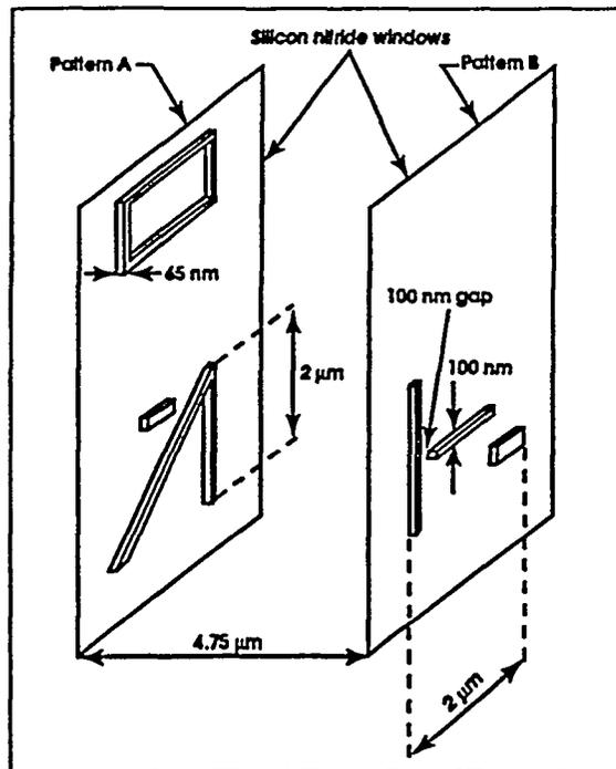
Fig. 2. Sketch of the 3-D microscopic test object. The two gold patterns were written using electron beam lithography.
