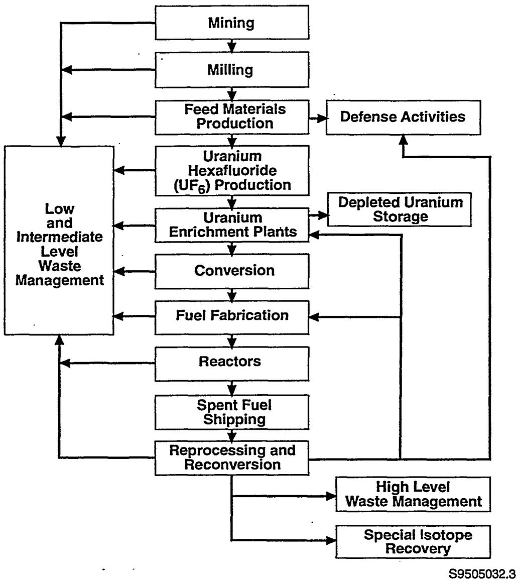
Figure 3. Waste generation in the nuclear fuel cycle.
