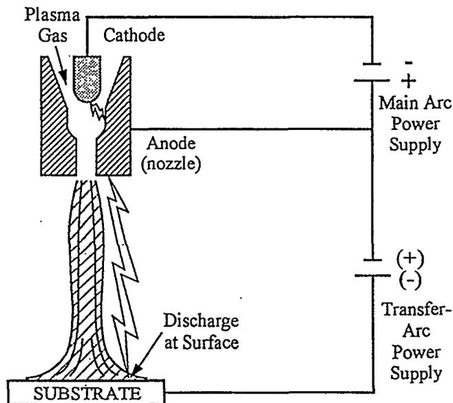
Fig. 1. Basic operation of negative transferred-arc cleaning.
