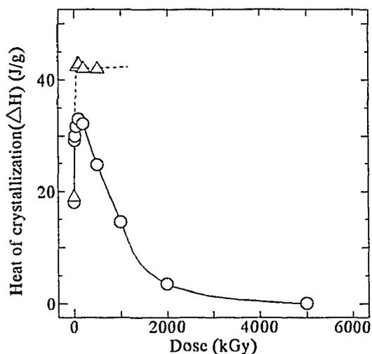
Fig.5 Heat of crystallization(ΔH) for PTFE irradiated in Ar gas at 340°C and at RT ; ○: irradiated at 340°C, △: irradiated at RT
