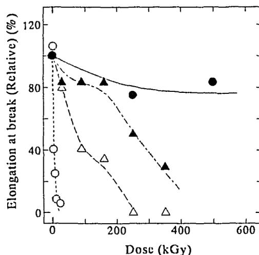
Fig.6 Elongation at break(relative) vs. dose  $\gamma$  irradiation in air for PTFE crosslinked with various conditions ;  $\circ$ :0kGy at 340°C,  $\triangle$ :300kGy at 340°C,  $\blacktriangle$ :500kGy at 340°C,  $\bullet$ : 2MGy at 340°C
