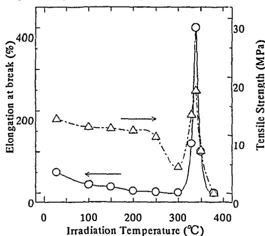
Fig.1 Irradiation temperature vs. mechanical properties for PTFE irradiated by electron beam to 100kGy in Ar gas
