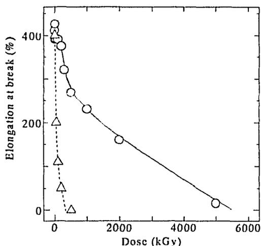
Fig.2 Elongation at break vs. dose for PTFE irradiated by electron beam in Ar gas at 340°C and at RT ; ○: irradiated at 340°C, △: irradiated at RT
