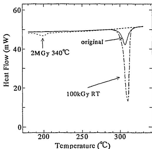
Fig.4 DSC thermograms of crystallization for PTFE irradiated in Ar gas at 340°C and at RT
