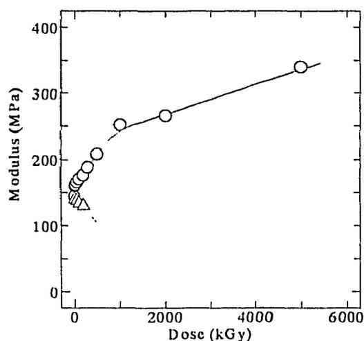
Fig.3 Modulus of PTFE irradiated by electron beam in Ar gas at 340°C and at RT ; ○: irradiated at 340°C, △: irradiated at RT
