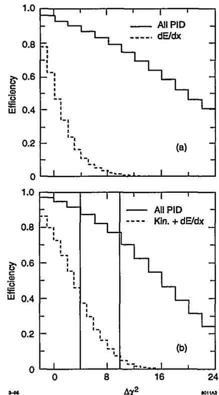
Fig. 3. The efficiency for accepting an event as a function of the  $\chi^2$  difference between events containing a  $(\pi^+\pi^-)$  hypothesis and those containing a kaon; the dashed line shows the simulated performance without the PID system, while the solid line adds the DIRC and forward ATC systems of  $B_{\text{ABAR}}$ : (a)  $B^0 \rightarrow \pi^+\pi^-$ . (b)  $B^0 \rightarrow \rho^+\pi^-$ .
