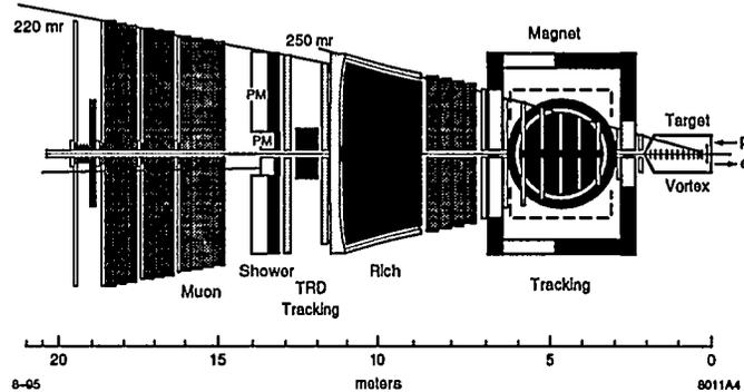
Fig. 15. Plan view of the HERA B detector.
