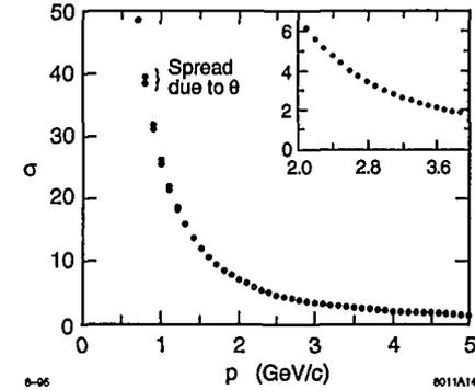
Fig. 14. Monte Carlo simulation of the  $K/\pi$  separation expected as a function of momentum for the Fast RICH at CLEO III. The spread in the points shows the separation range due to different values of the track polar angle. The inset shows the high momentum region magnified.
