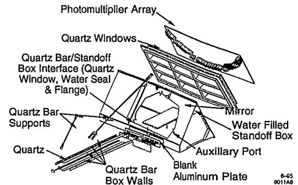
Fig. 8. Isometric view of the Prototype-II detector.
