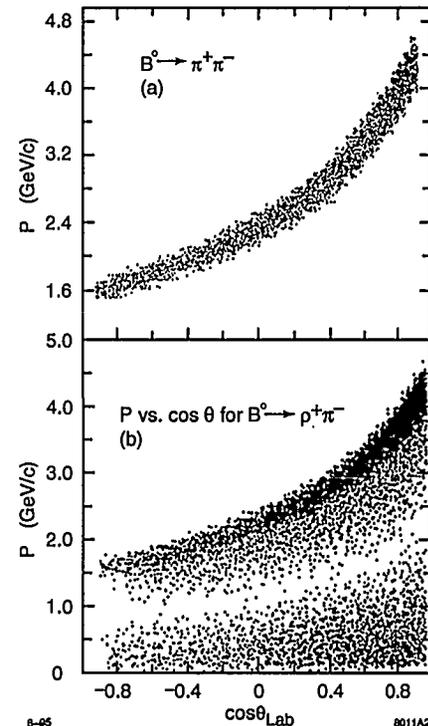
Fig. 2. (a) The momentum spectrum vs. the cosine of the laboratory angle for pions from the reaction  $B^0 \rightarrow \pi^+\pi^-$ . (b) The momentum spectrum vs. the cosine of the laboratory angle for charged pions from the reaction  $B^0 \rightarrow \rho^+\pi^-$ .
