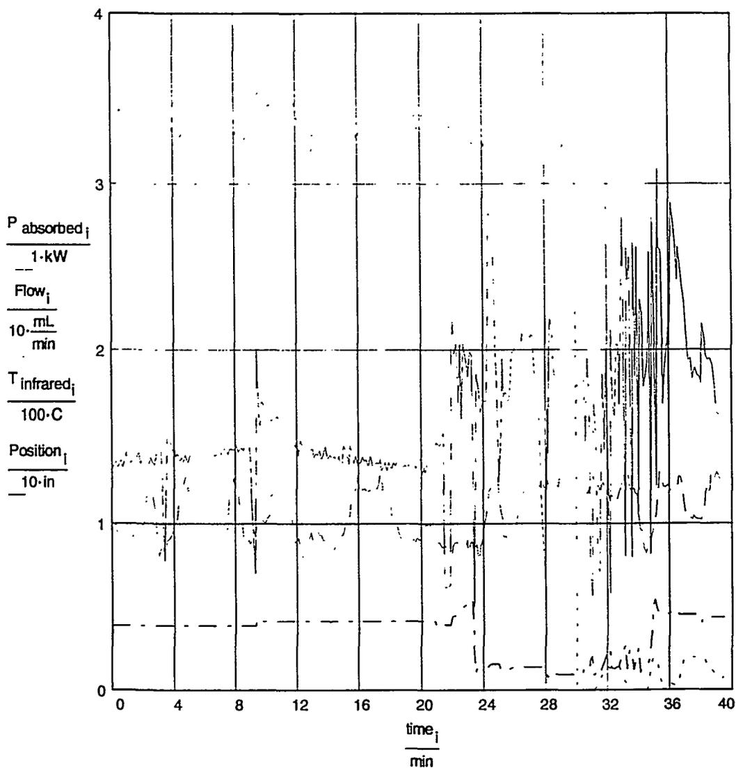
Fig. 3. Absorbed power, flow, infrared temperature and tuning position versus time (all parameters normalized as shown).
