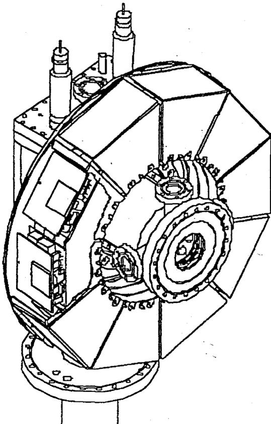
Figure 9. Half-lattice module with induction cell and modulator.
