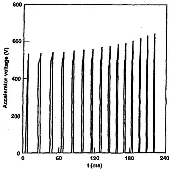
Figure 6. Combined waveform including acceleration and longitudinal confinement.
