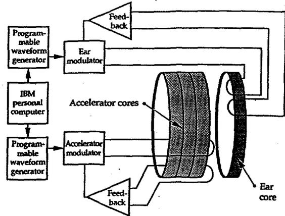
Figure 7. Block diagram induction cell modulator for small-scale recirculator.
