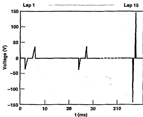
Figure 5. Example of longitudinal confinement pulses required for small recirculator.
