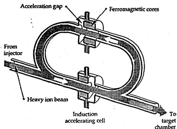
Figure 1. A recirculator utilizes the same accelerator components multiple times.
