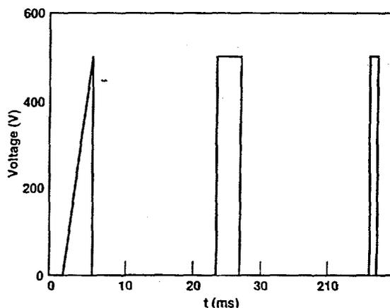
Figure 4. Illustration of range of pulse shapes that must be generated by induction cell modulators.
