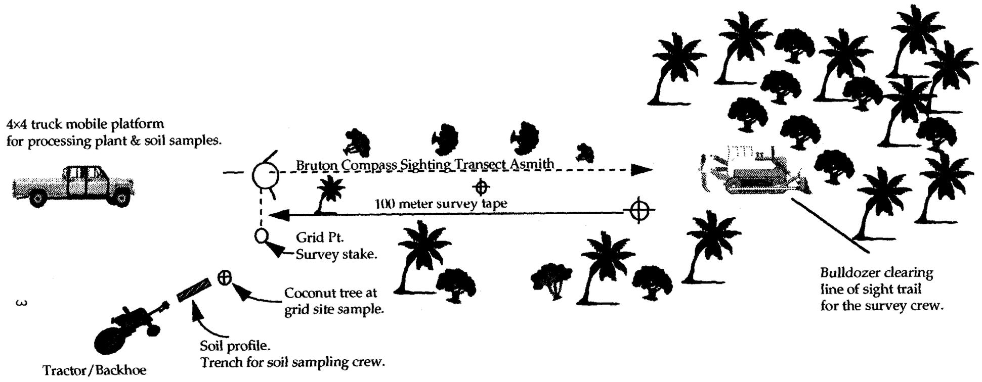
Figure 1. Grid Equipment Field Deployment.
