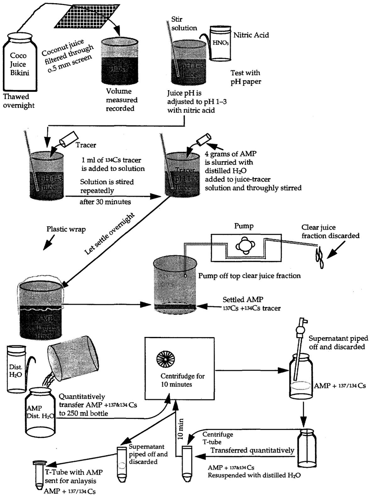
Figure 6. Coconut juice processing procedures flow diagram.
