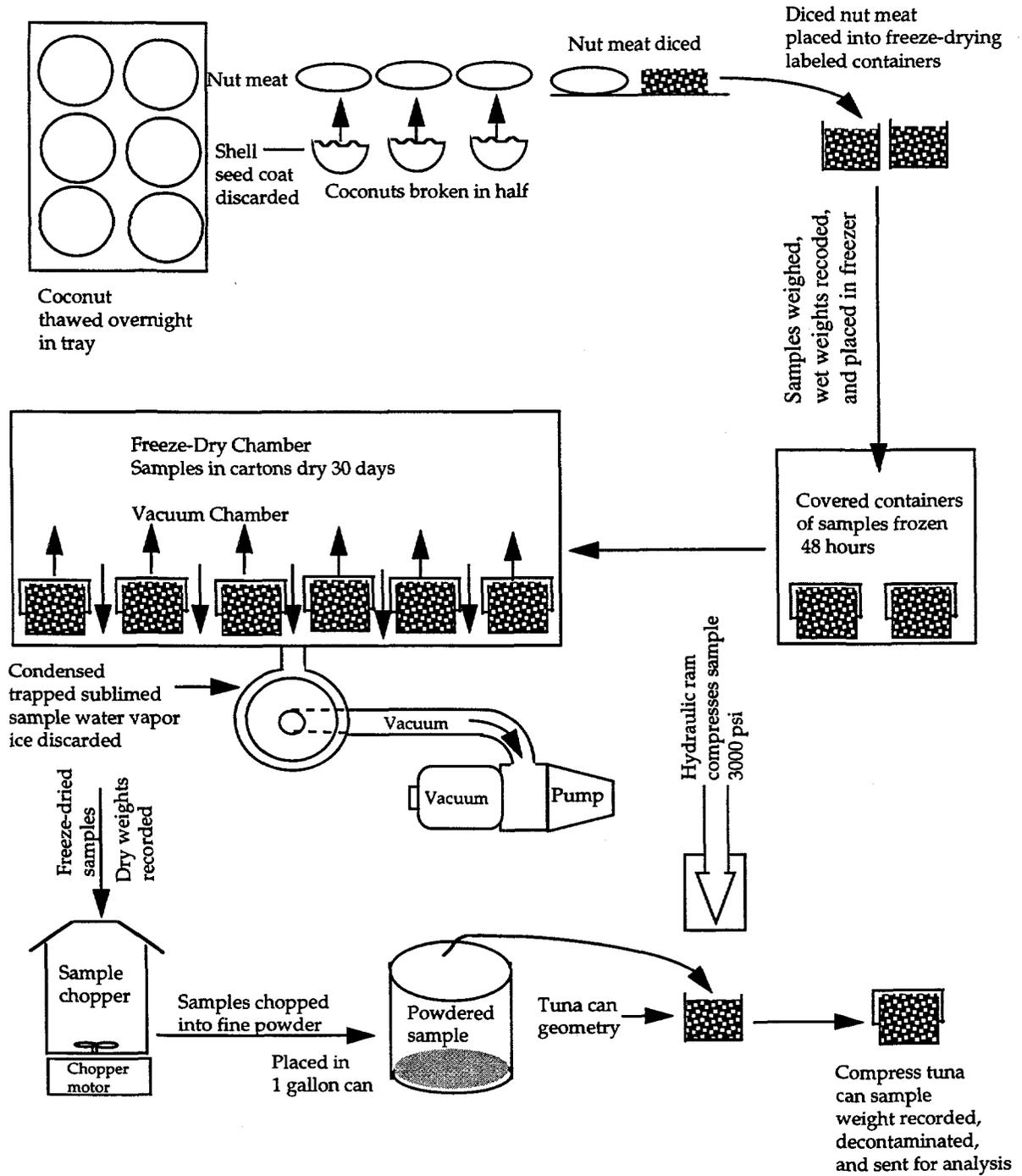
Figure 4. Laboratory flow diagram of edible vegetation sample processing procedure.
