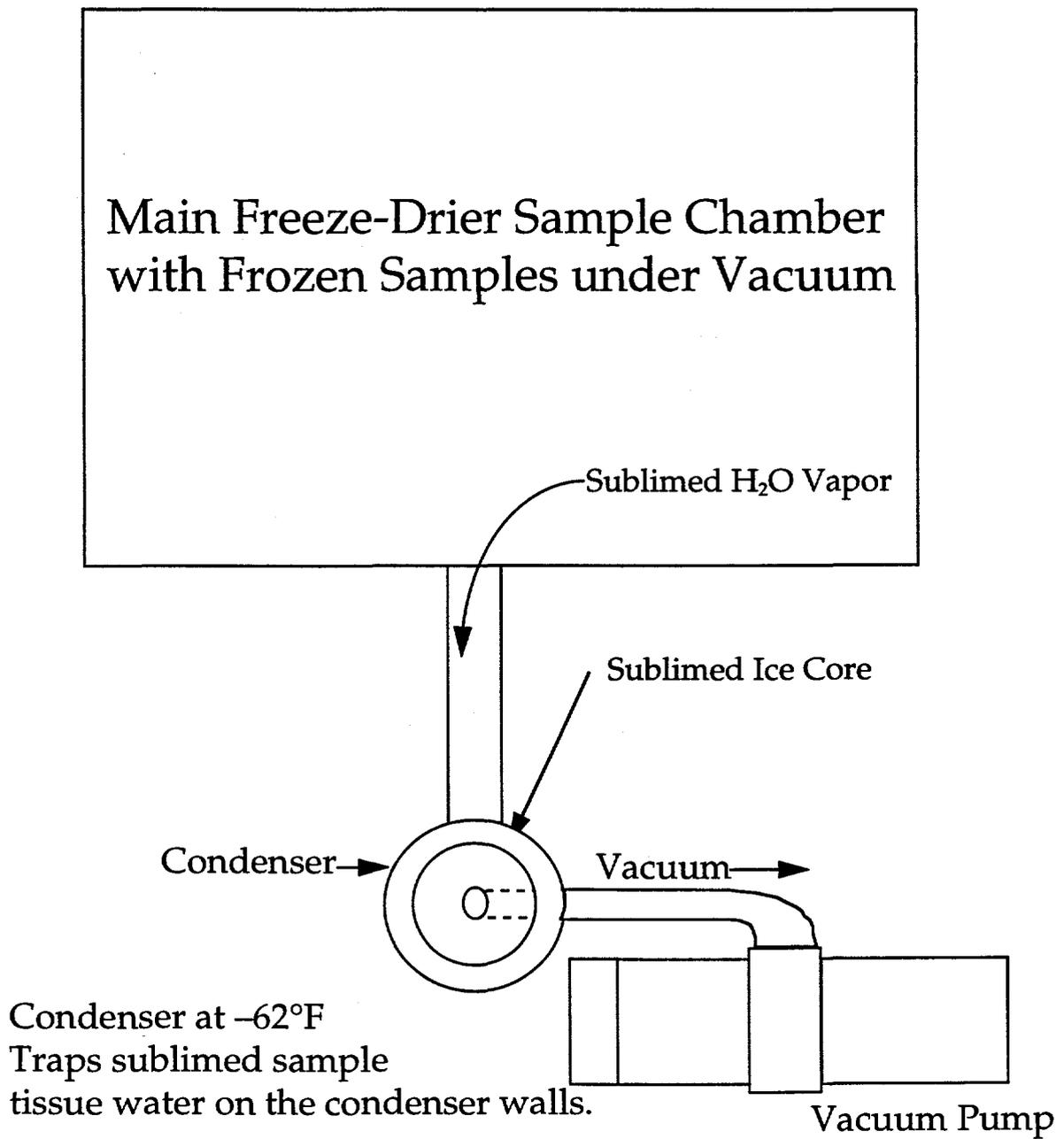
Figure 5. Northstar freeze-dryer.
