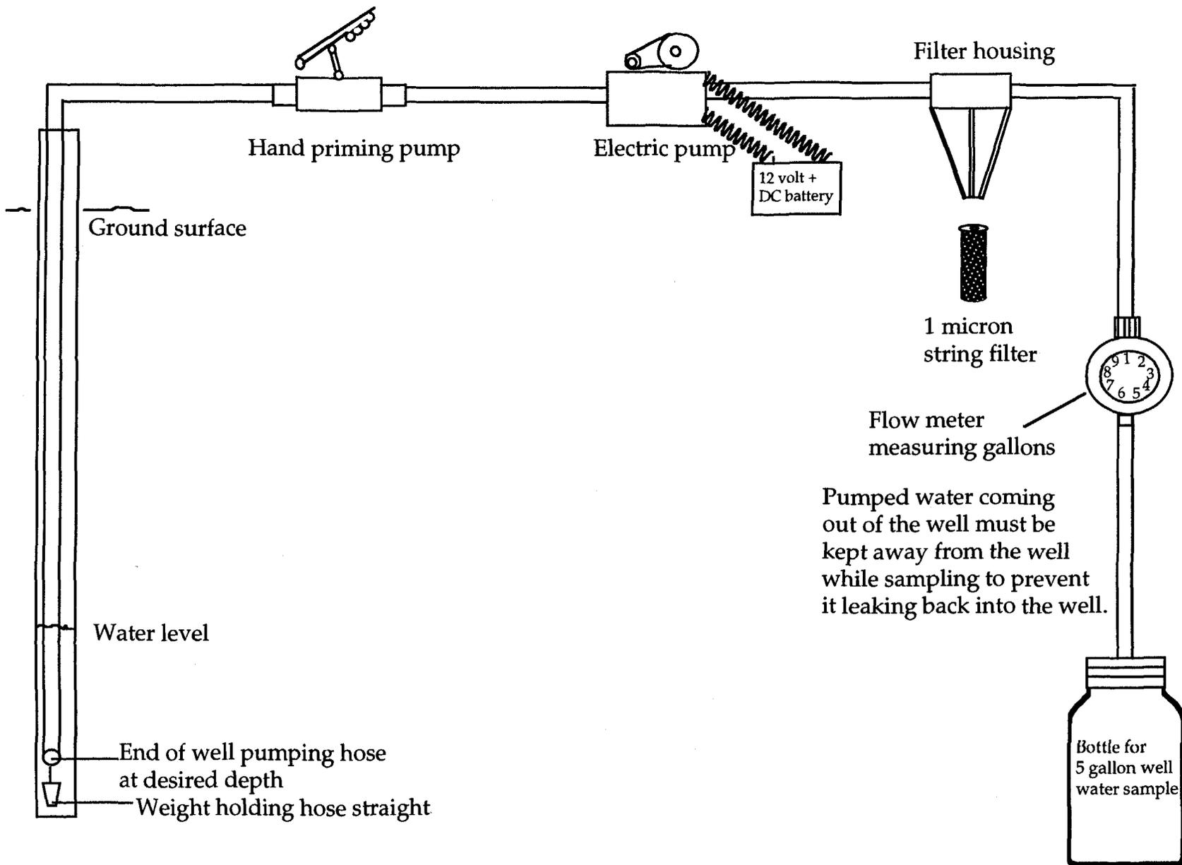
Figure 3. Well pumping array.
