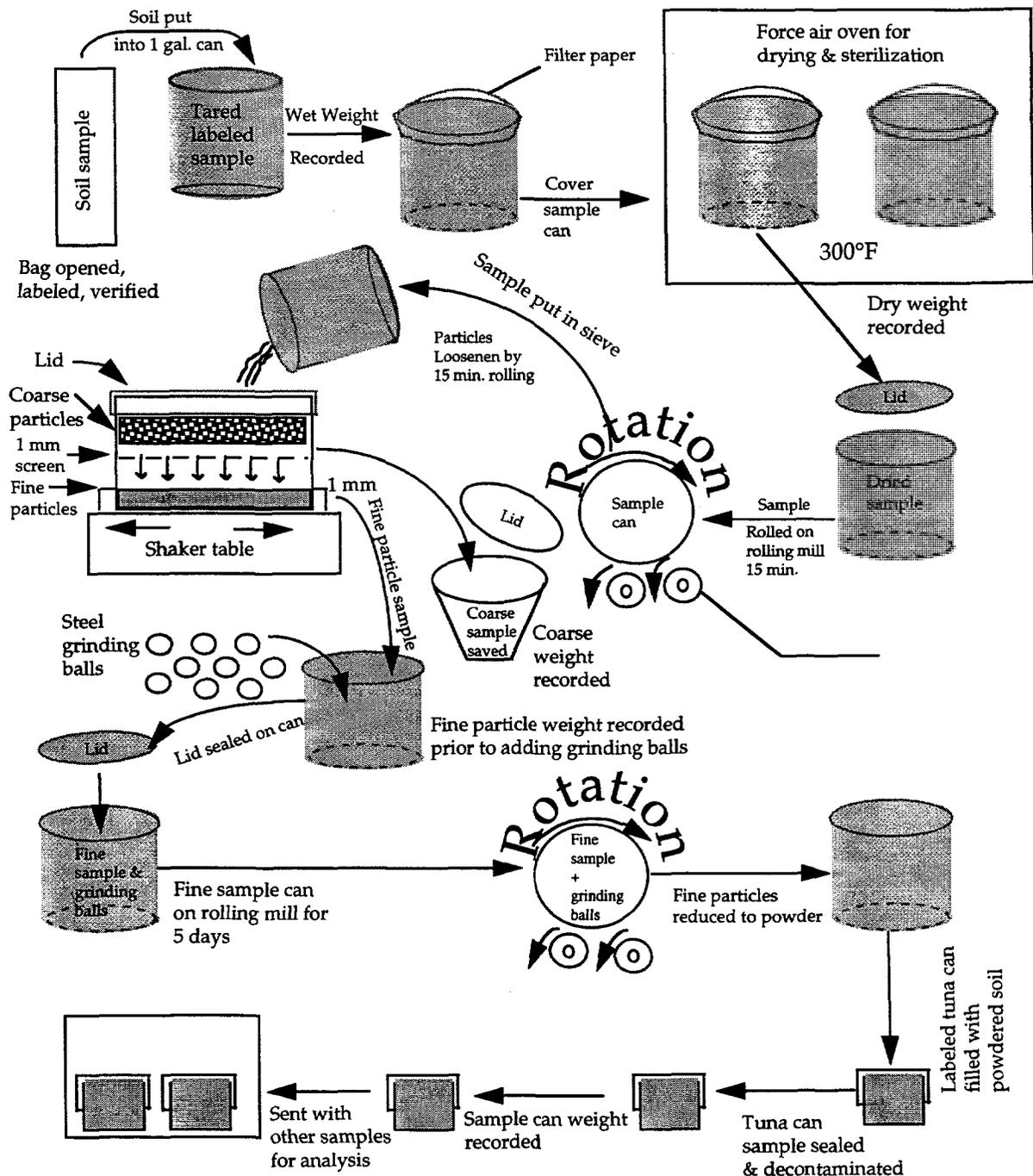
Figure 7. Soil sample processing procedures flow diagram.
