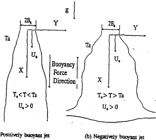
Figure 8 Schematic of a positively and a negatively buoyant jet.
