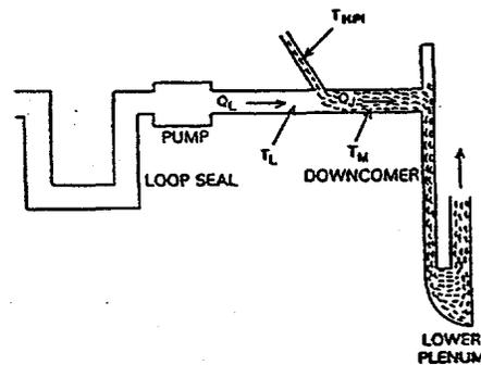
Figure 7 Conceptual representation of the well-mixed condition<sup>19</sup>
