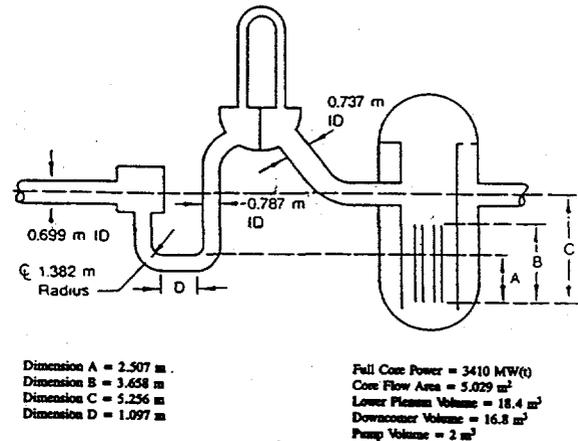
Figure 2 Pertinent data for a typical Westinghouse design Four-Loop Plant (RESAR-3S)
