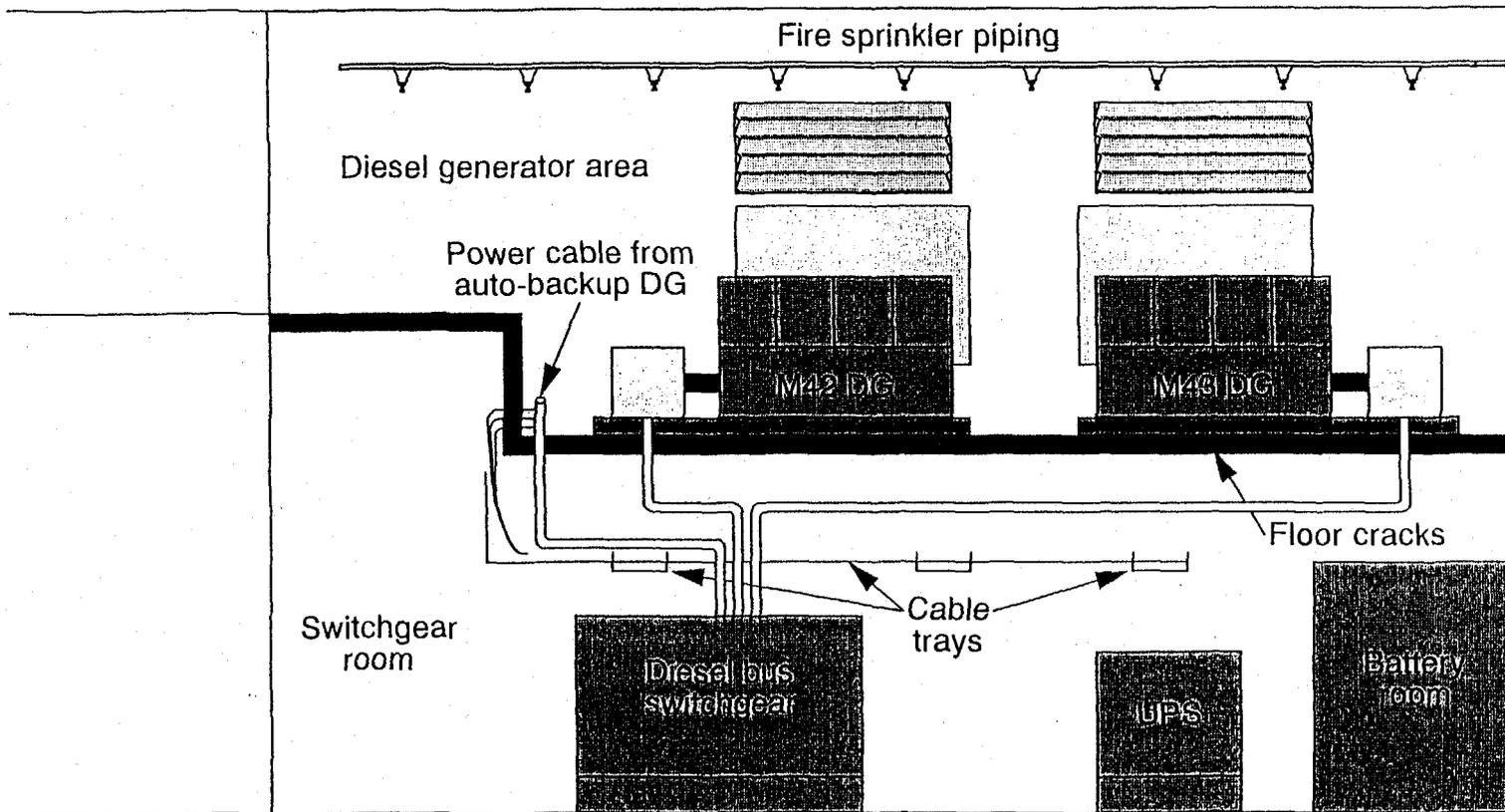
FIGURE 2. DIESEL PIT FLOOD PROPAGATION PATHS
