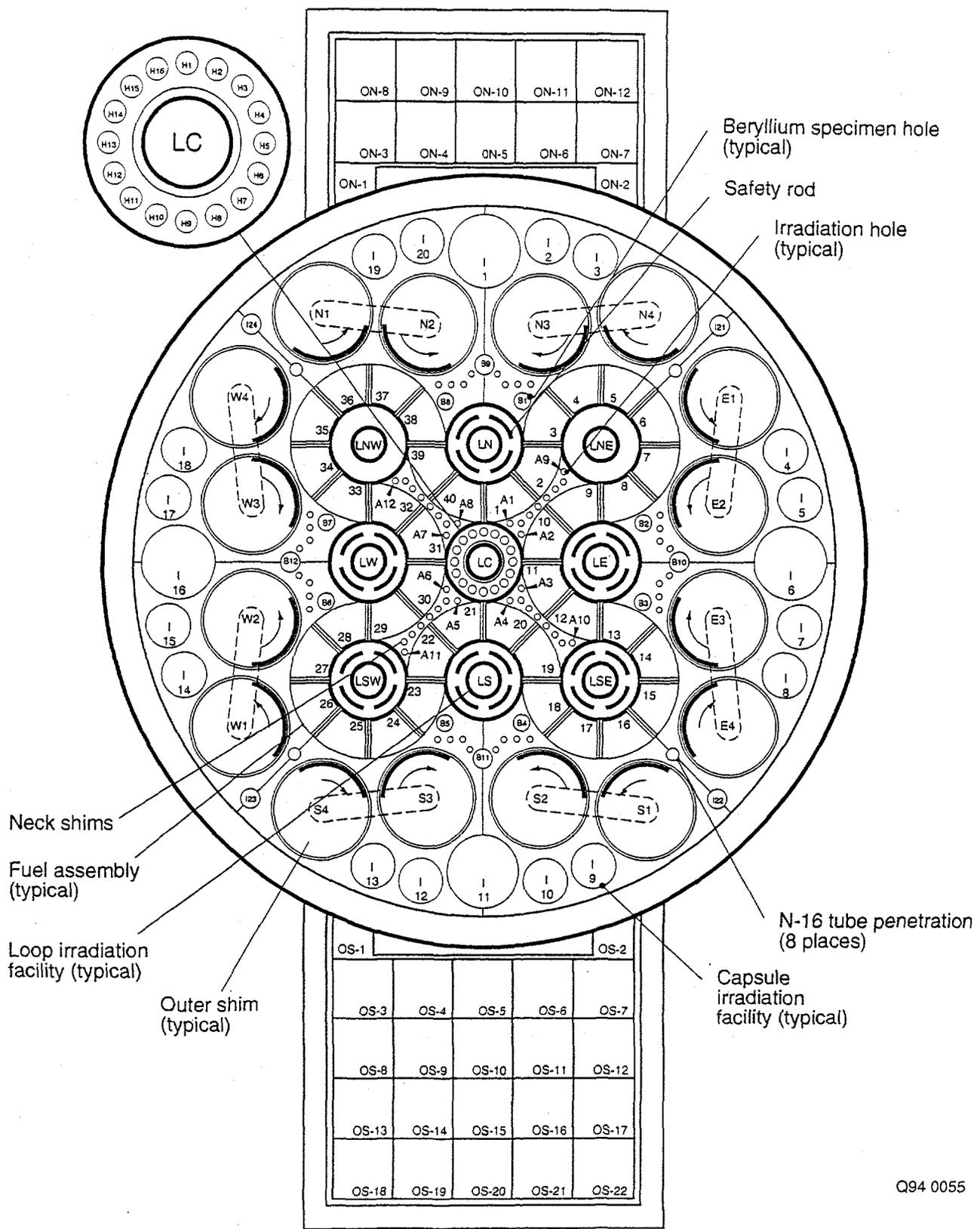
FIGURE 1. HORIZONTAL CROSS SECTION OF ATR CORE
