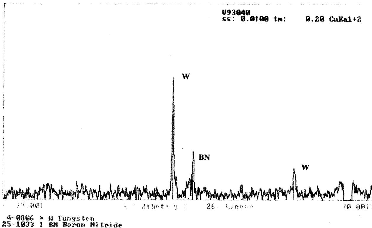
Figure 9: X-Ray diffraction analysis of specimen PP93-40
