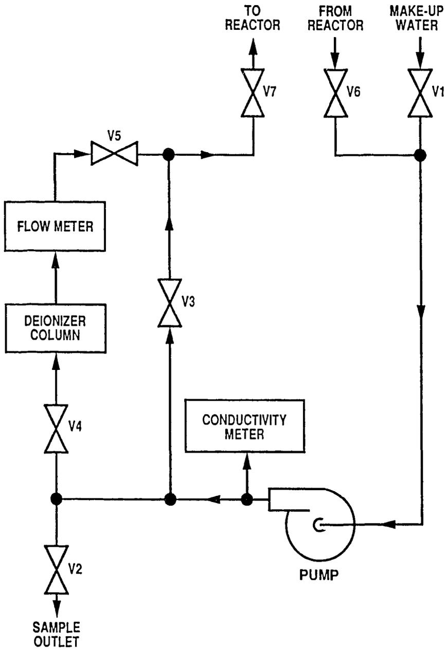
Figure 6: Reactor container water flow diagram.
