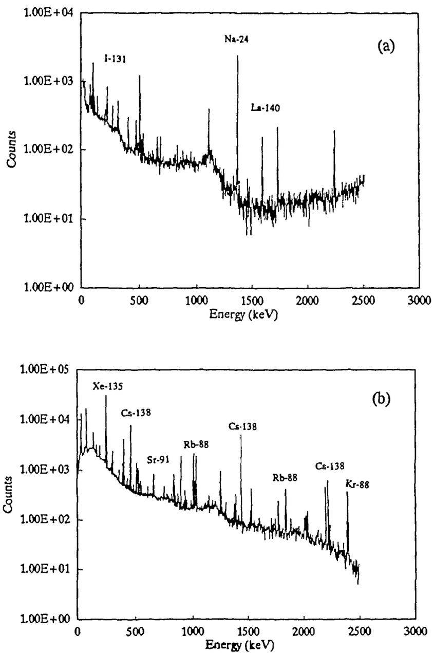
Figure 9: Gamma ray spectrum for the reactor container water.
