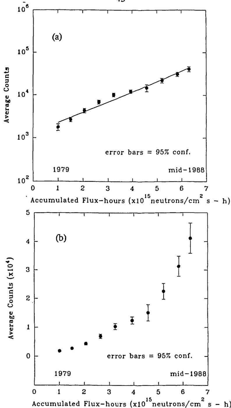
Figure 16: The weekly activity concentration of Xe-133 (averaged over a year) in the SLOWPOKE-2 reactor at Ecole Polytechnique versus the accumulated flux hours. (The concentration has been recorded as part of the routine maintenance at this facility.) Inspection of the semi-log plot (a) and the linear plot (b) indicate that the Xe-133 activity concentration varies as a non-linear phenomenon with burnup. (The error bars indicate 95% confidence limits.)
