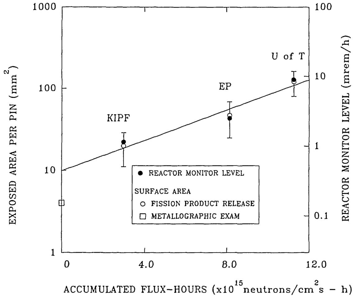
Figure 15: Increasing exposed fuel and alarm levels with burnup for U of T, EP and KIPF reactors. (The error bars indicate 95% confidence limits.)
