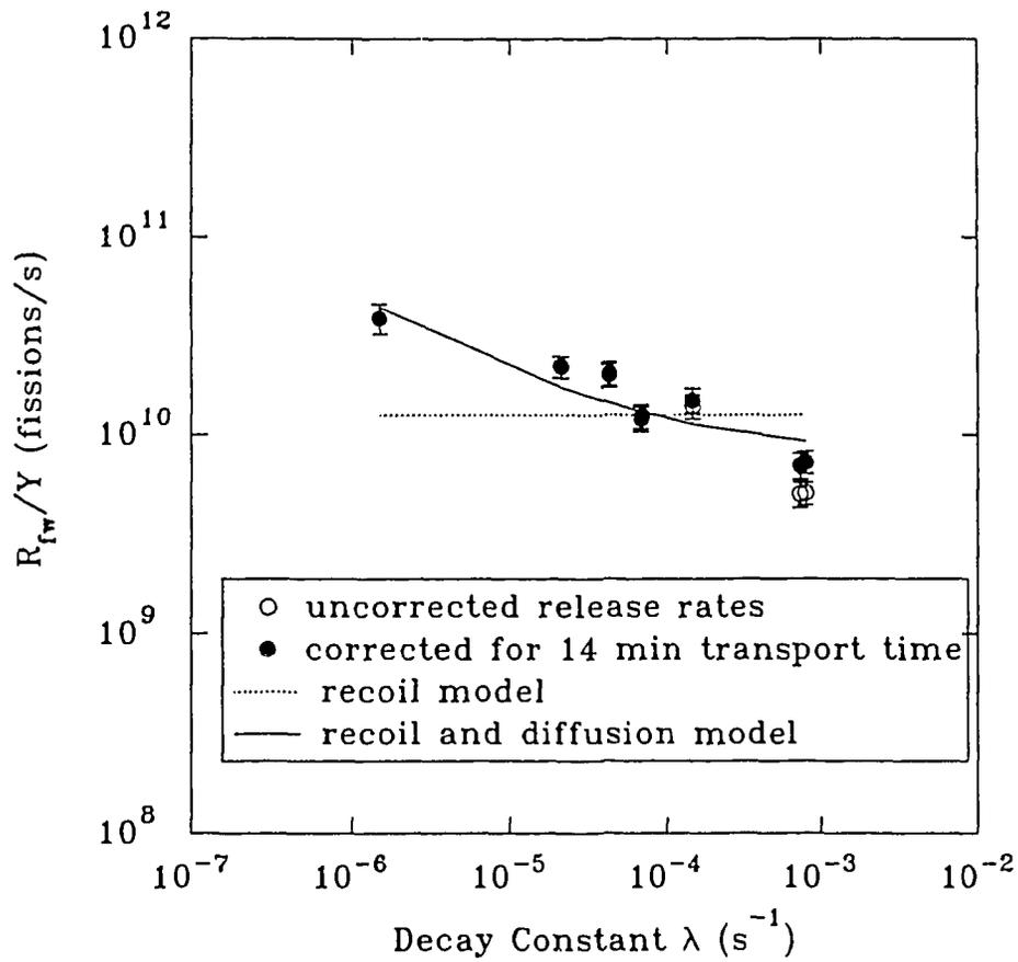
Figure 13(b):  $R_w/Y$  versus  $\lambda$  plot for EP reactor.
