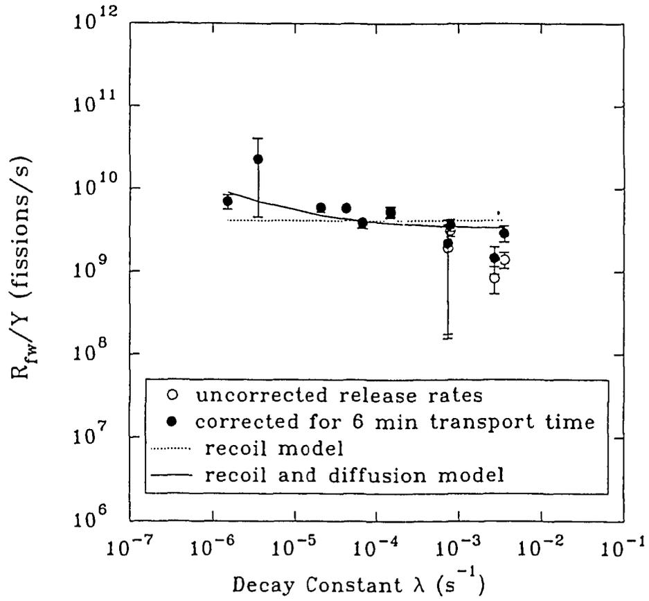
Figure 13(c):  $R_{fw}/Y$  versus  $\lambda$  plot for KIPF reactor.
