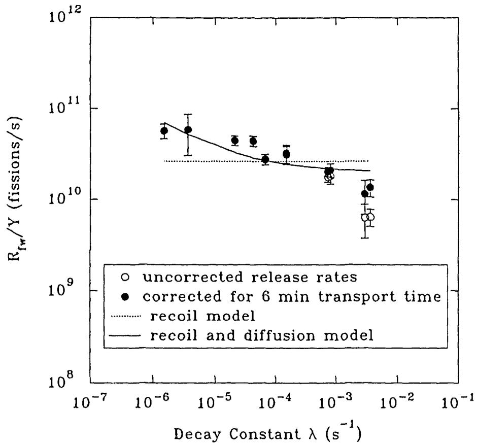
Figure 13(a):  $R_{fr}/Y$  versus  $\lambda$  plot for U of T reactor.
