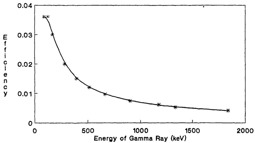
Figure 10: Detector efficiency curve for the GMX high purity germanium detector.
