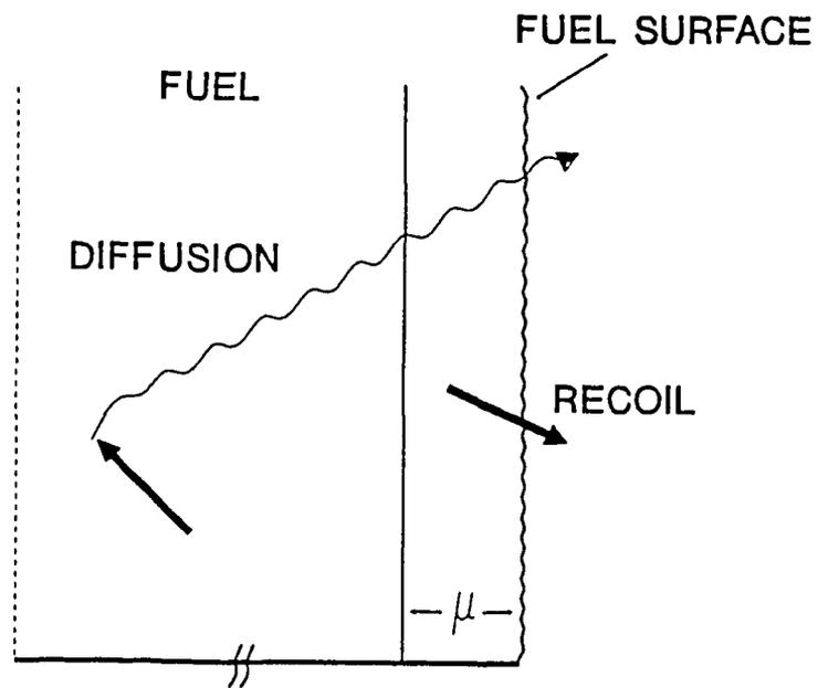
Figure 12: Schematic of diffusion and recoil release processes.
