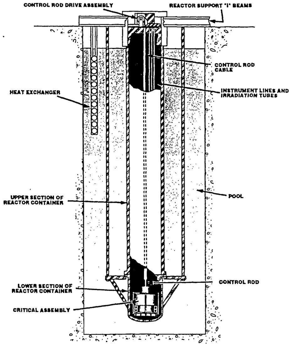
Figure 2: Reactor general assembly. (Taken from Reference 2.)
