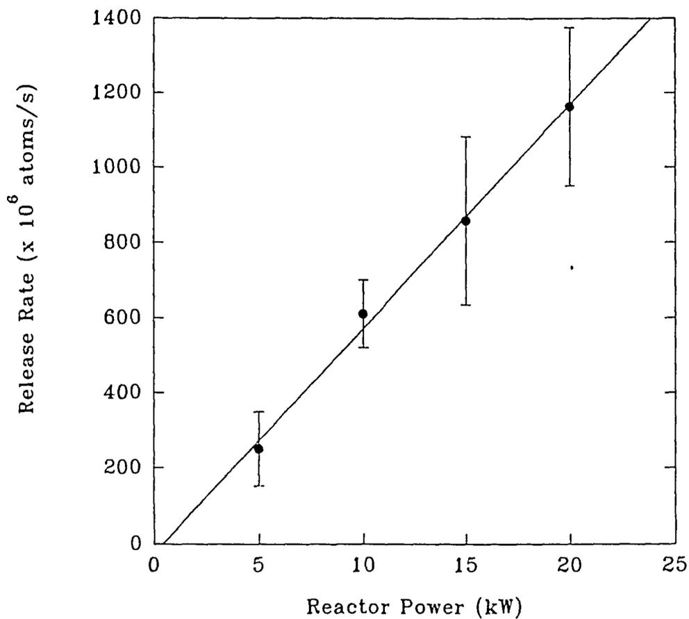
Figure 14: Release rate of  $^{136}\text{Xe}$  (fuel-to-water) at KIPF reactor as a function of reactor power. (The error bars indicate 95% confidence limits.)
