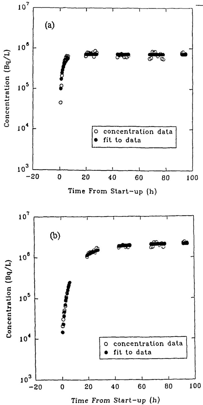
Figure 11: The concentration of (a) Kr-88 and (b) Xe-135 in the U of T reactor container water.
