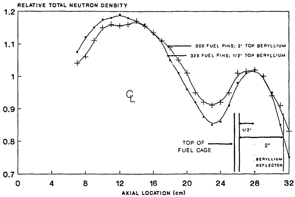
Figure 18 : Axial neutron flux distribution of a SLOWPOKE-2 reactor with 1/2" and 2" of beryllium added to the upper shim tray. (Taken from Reference 2.)
