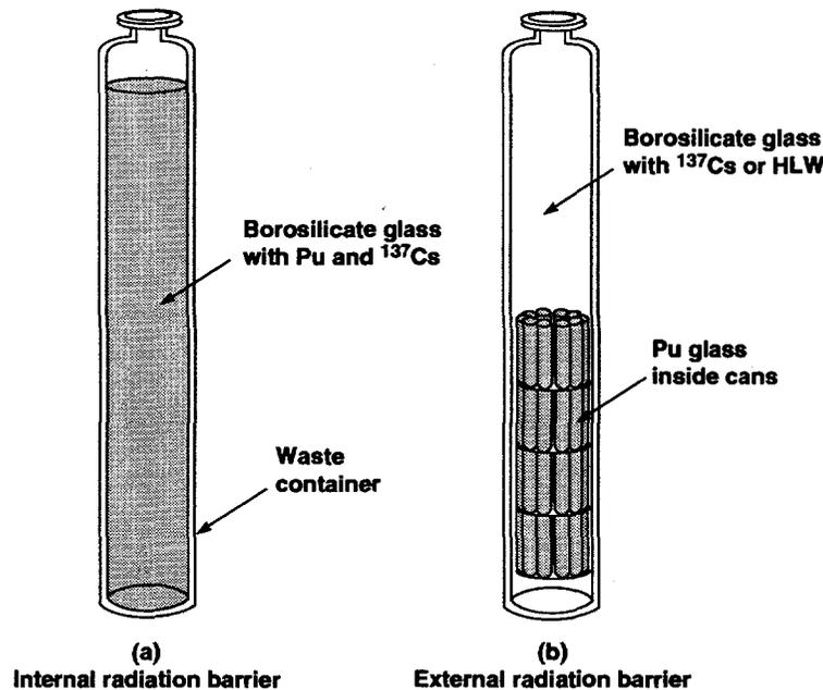
Figure 3. Two options for vitrification of Pu.
