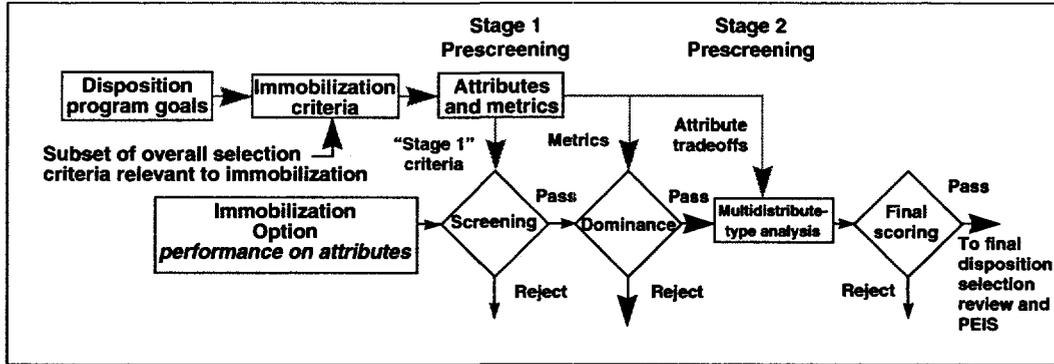
Figure 2. Pu immobilization prescreening process.
