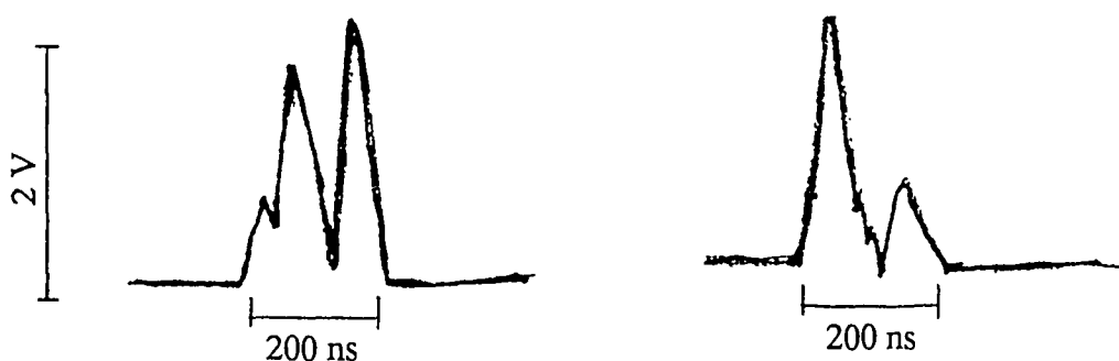
Fig.2. PIN diode X-ray signals: a) D_2 - filling, b) Ne - filling.
