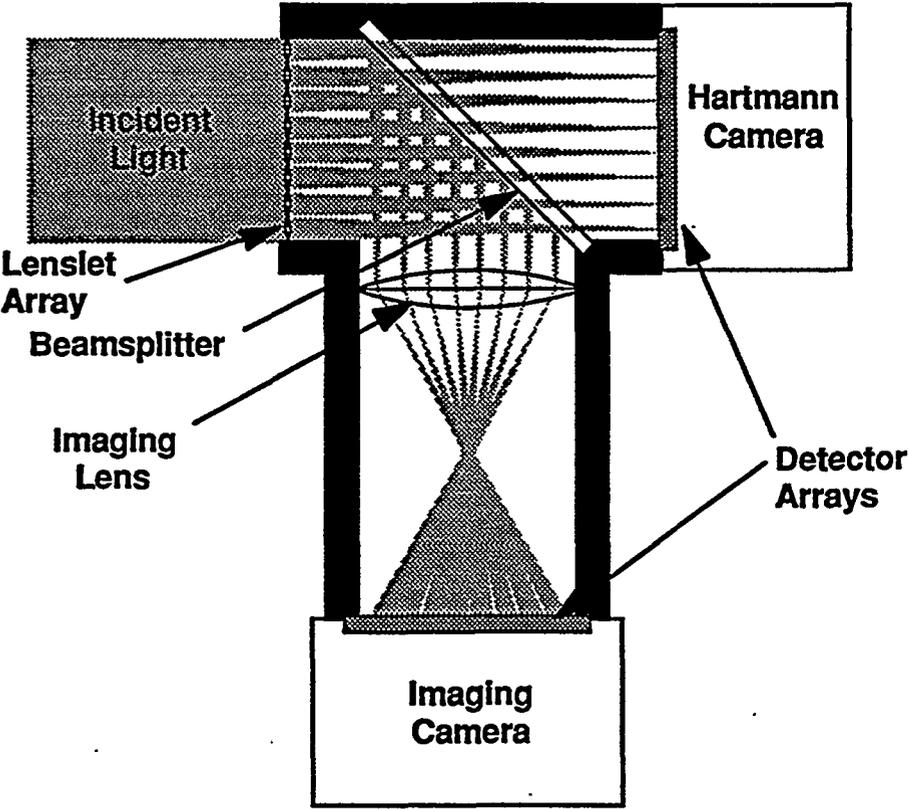
Fig. 3 Schematic of Hartmann sensor showing the two video cameras for data and alignment.
