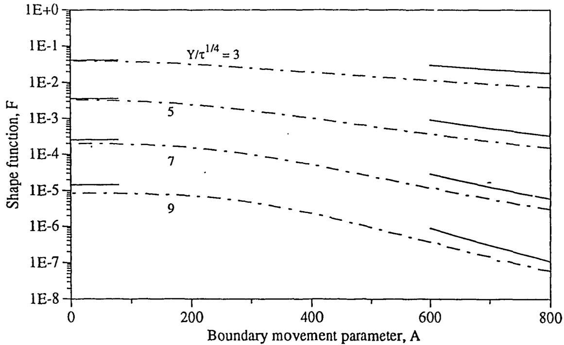
Figure 1. Shape function for solute penetration of a polycrystalline solid with a moving boundaries. Dot-dash curves: approximate solution of ref. [7]; horizontal solid lines: Whipple solution for  $A=0$ ; and solid curves: Glaeser-Evans solution for  $A \rightarrow \infty$ . The dimensionless time  $\tau$  is  $10^{-4}$ ; for various time-depth variables  $Y/\tau^{1/4}$ .
