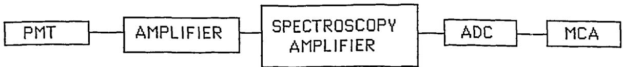
Fig. 19. A schematic view of the electronic set-up for pulse height measurements.
