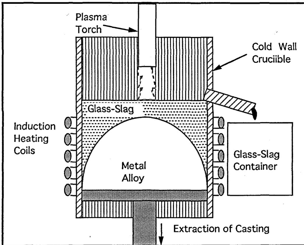
Figure 2. Hybrid Plasma/Induction Cold Crucible Melting System
