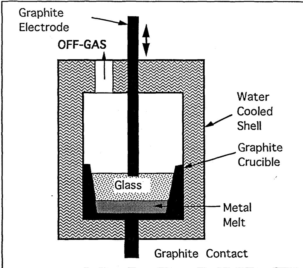
Figure 1 Electro-Pyrolysis Inc. DC Graphite Arc Melter
