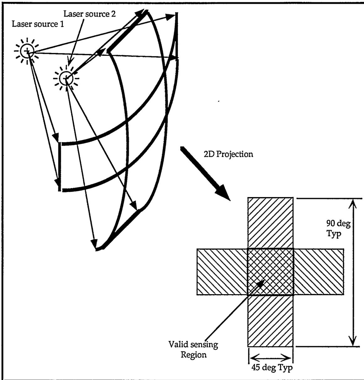
Fig. 1 Pan-and-tilt laser scanners work area.
