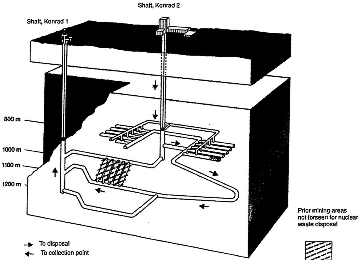
**Figure 5.** Schematic of Konrad repository (courtesy of BfS).
