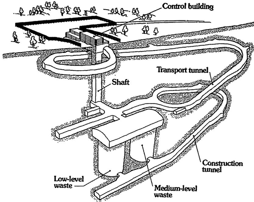
Figure 2. The VLJ repository operated by TVO (courtesy of TVO).
