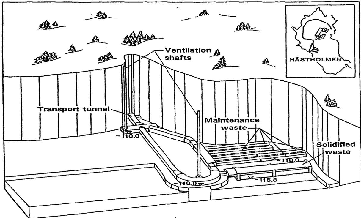
Figure 3. The low- and medium-level waste repository at Hästholmen Island, City of Loviisa. The repository is being constructed for IVO (courtesy of TVO).
