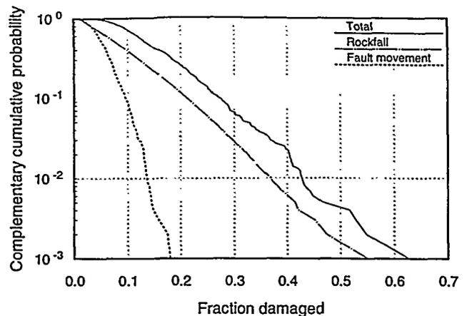
Figure 2. Distribution of the fraction of containers potentially damaged by rockfall and by fault displacement within one million years. (Some of these containers might fail by corrosion before being damaged by rockfall.)
