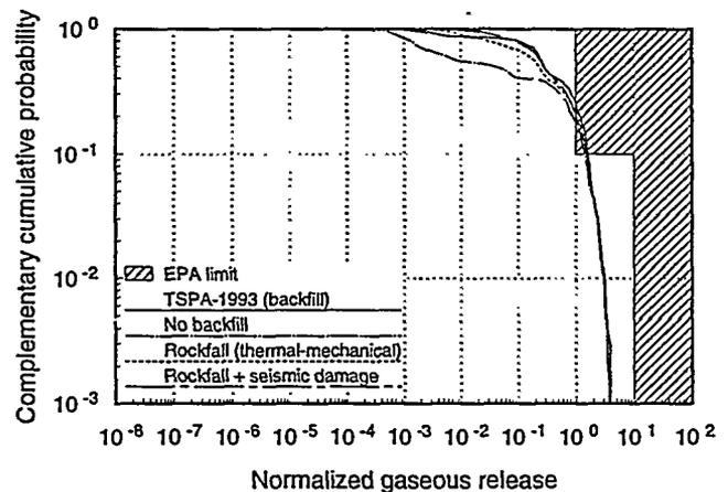
Figure 8. Distributions of 10,000-yr normalized cumulative gaseous release for the composite-porosity model.
