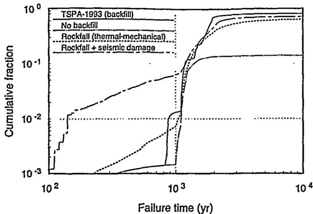
Figure 6. Mean container-failure distributions for the composite-porosity model.
