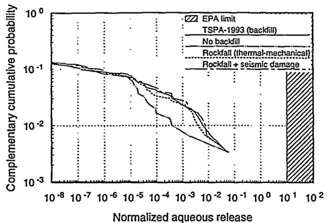
Figure 7. Distributions of 10,000-yr normalized cumulative aqueous release for the composite-porosity model (Column 8 only).
