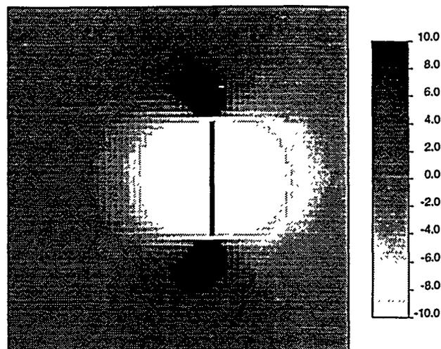
Figure 4. Map view of changes in strain calculated for a 10-km rupture displaced 1 m along a normal fault dipping  $60^\circ$  W. Area depicted is 30 km by 30 km. Scale shows volumetric strain (times  $10^6$ ). Light areas indicate compression; dark areas indicate tension.
