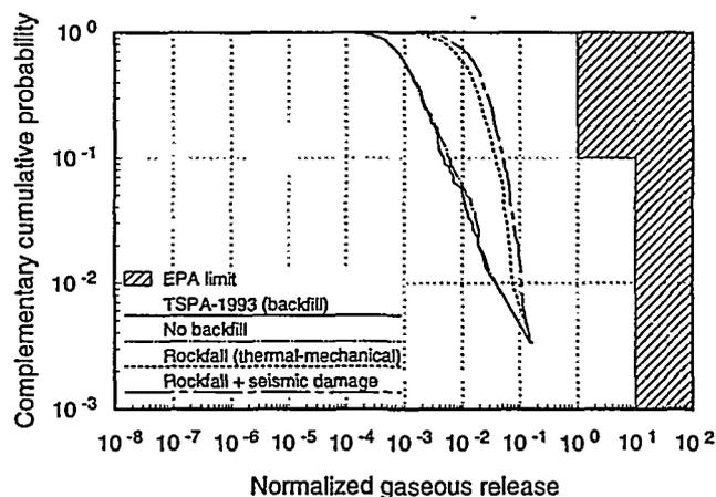
Figure 11. Distributions of 10,000-yr normalized cumulative gaseous release for the weeps model.
