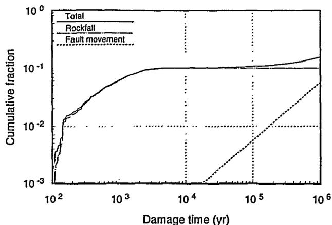
Figure 3. Mean distribution of the time at which containers are potentially damaged by rockfall and by fault displacement (some containers might fail by corrosion first). The rockfall distribution includes both rockfall due to thermal-mechanical stresses and earthquakes.
