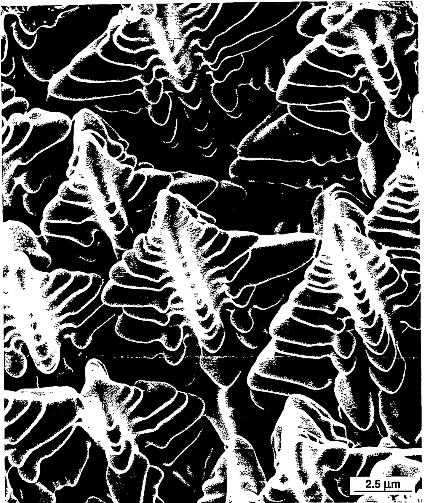
**Fig. 3** Scanning electron micrograph showing the development of dendrites in a nickel-based superalloy single-crystal weld.
