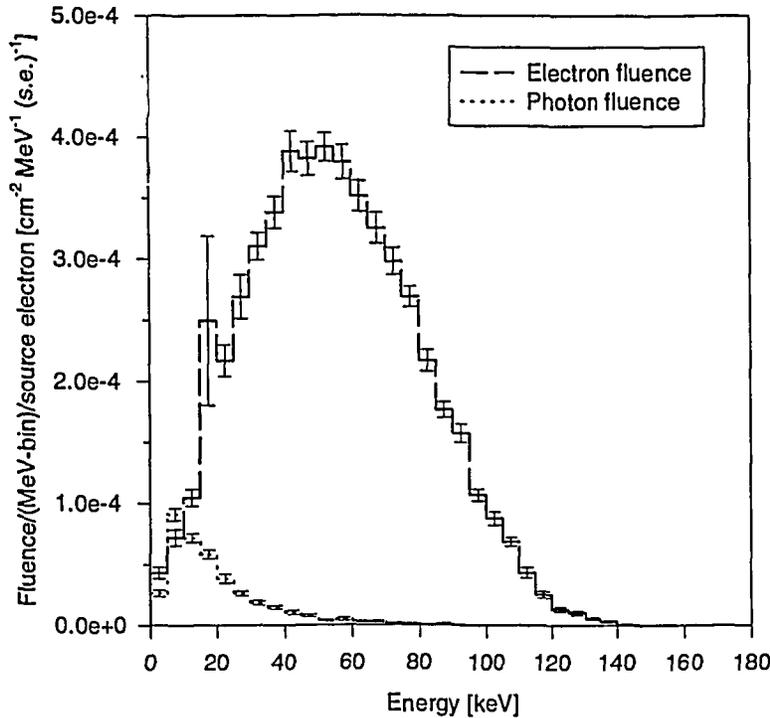
Figure 7. MC calculated on-axis fluence at 50 mm distance in air from the source surface in 5 keV bins. Average energies are 55 keV for electrons and 20 keV for photons.
