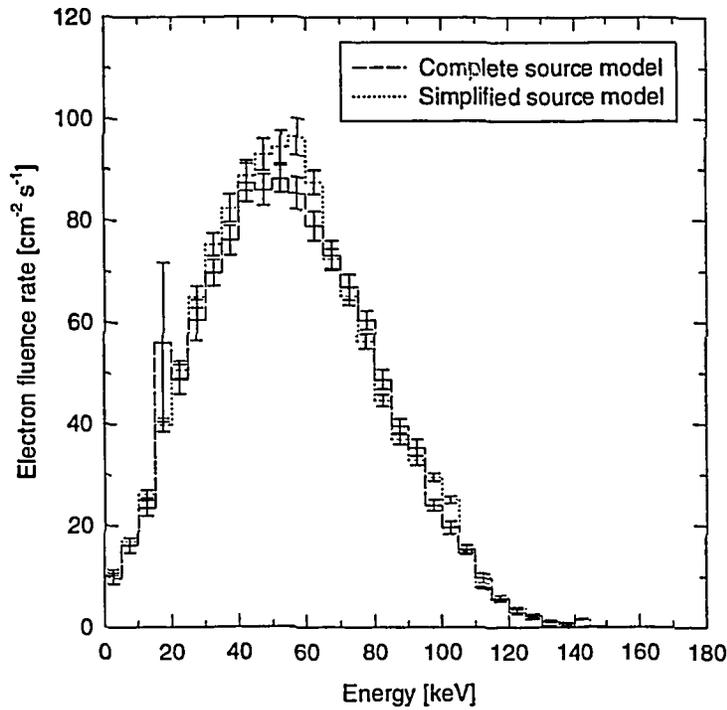
Figure 10. Calculated on-axis electron fluence rate spectra in air at 50 mm distance from the source surface. The spectra were calculated for a region with 25 mm radius. Average energies are 55 keV for both complete and simplified source.
