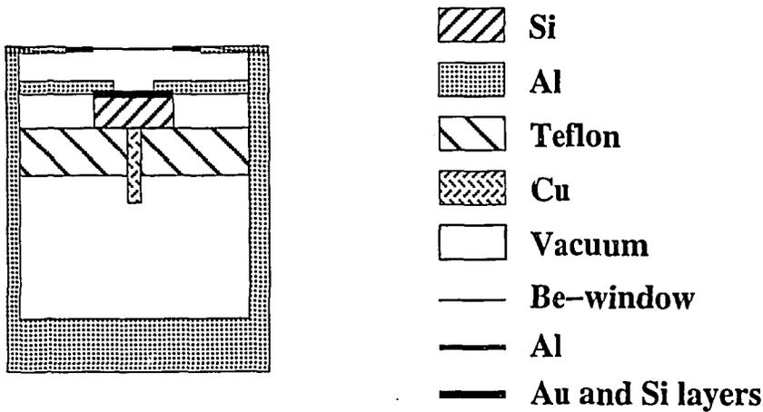
Figure 2. Cross section of the Si(Li) detector model.
