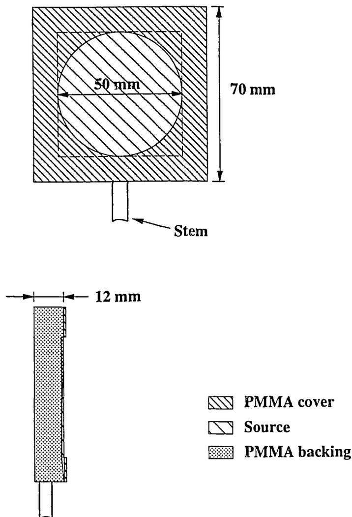
Figure 4. Configuration of physical source including source holder (backing and cover) of PMMA.
