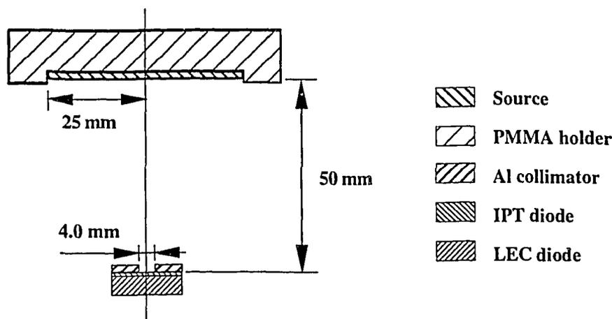
Figure 1.  $^{14}\text{C}$  source and  $\beta$  spectrometer consisting of two Si detectors.
