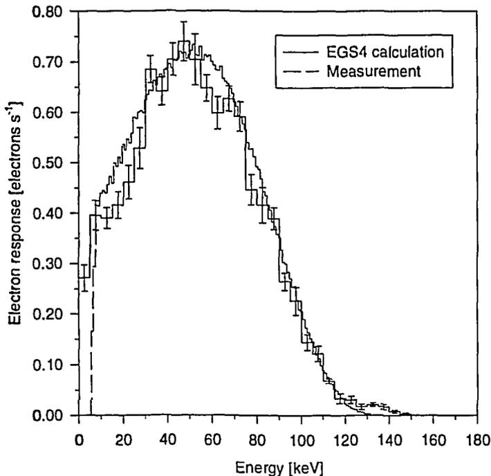
*Figure 13. Measured and calculated electron response as a function of energy for the Si(Li) detector. The calculated response in 5 keV bins is divided by 5 to make it comparable with the measured response in 1 keV bins. Furthermore, the calculated response is multiplied by the ratio of measured electrons to calculated electrons ( $53/194 = 0.27$ ) to compare the shapes of the energy spectra. Average energies are 52 keV and 53.3 keV for calculated and measured response, respectively.*
