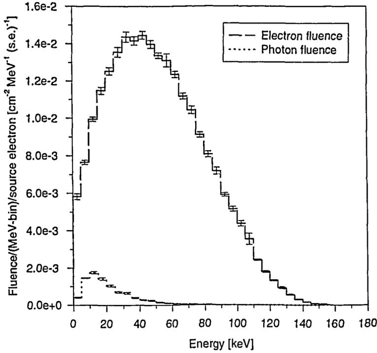
Figure 6. The MC calculated fluence at source surface in 5 keV bins. Average energies are 52 keV for electrons and 22 keV for photons.
