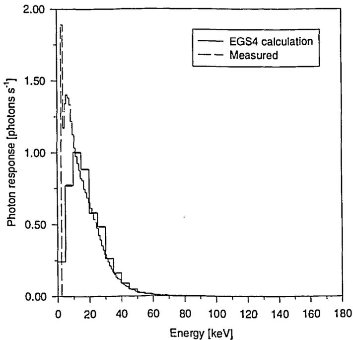
Figure 15. Measured and calculated photon response as a function of energy for the Si(Li) detector. The calculated response in 5 keV bins is divided by 5 to make it comparable with the measured response in 1 keV bins.
