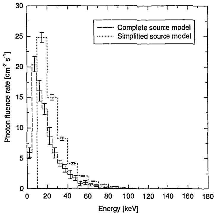
Figure 11. Calculated on-axis photon fluence rate spectra in air at 50 mm distance from the source surface. The spectra were calculated for a region with 25 mm radius. Average energies are 25 keV and 27 keV for complete and simplified source, respectively.
