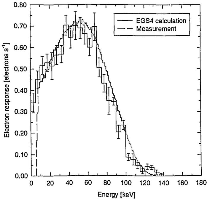
Figure 14. Comparison of measured and calculated electron response as a function of energy for the Si(Li) detector assuming a Si deadlayer 12  $\mu\text{m}$  thick. The calculated response in 5 keV bins is divided by 5 to make it comparable with the measured response in 1 keV bins. Furthermore, the calculated response is multiplied by the ratio of measured electrons to calculated electrons ( $53/69 = 0.77$ ) to compare the shapes of the energy spectra.
