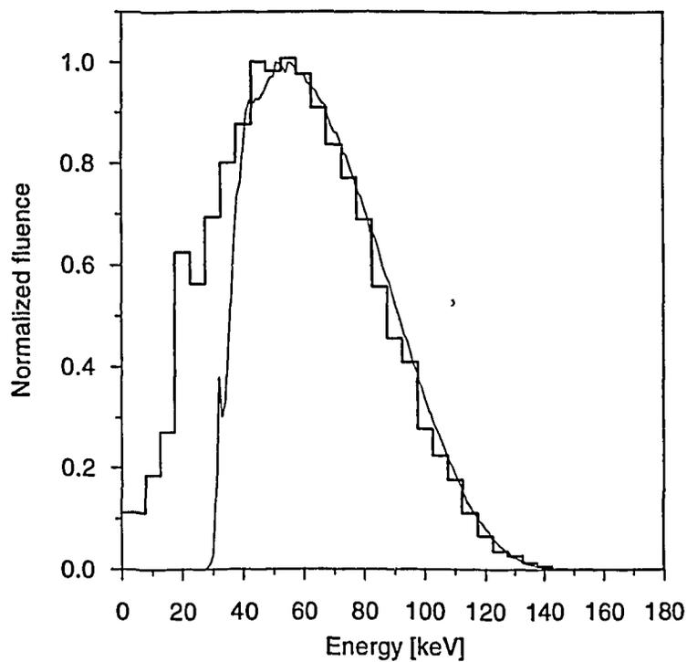
Figure 9.  $^{14}\text{C}$  spectrum measured at 50 mm distance in air at CEA, France. Average energy is 67 keV. The spectrum is normalized to peak at 1. The histogram shows the calculated energy spectrum also normalized to peak at 1. For uncertainties associated with the histogram, see Fig. 7.
