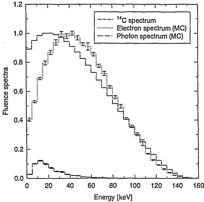
Figure 8. The spectrum for the  $^{14}\text{C}$  radionuclide and the MC calculated fluence spectra for electrons and photons at the source surface shown in 5 keV bins. Average  $\beta$  energy for the radionuclide is 49 keV, and for the MC calculated spectra 52 keV for electrons and 22 keV for photons. The electron spectra are normalized to the peak values for comparison. The photon spectrum has been multiplied by the same normalization factor as the MC calculated electron spectrum.
