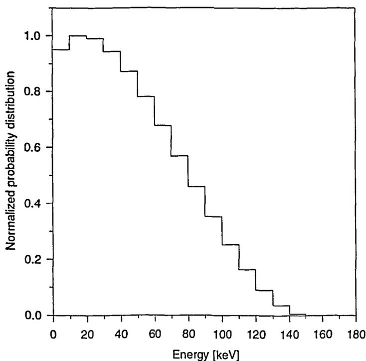
Figure 3. Spectrum for the  $^{14}\text{C}$  radionuclide calculated in 10 keV bins.
