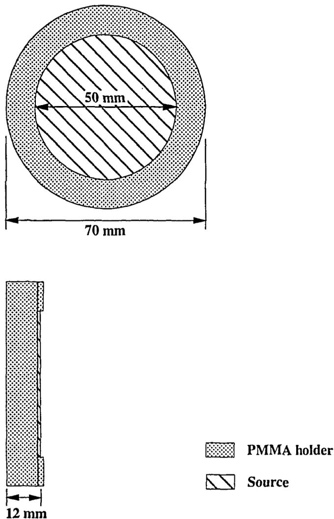
Figure 5. Configuration of complete model of  $^{14}\text{C}$  source for calculations including source holder (backing and cover) made of PMMA.
