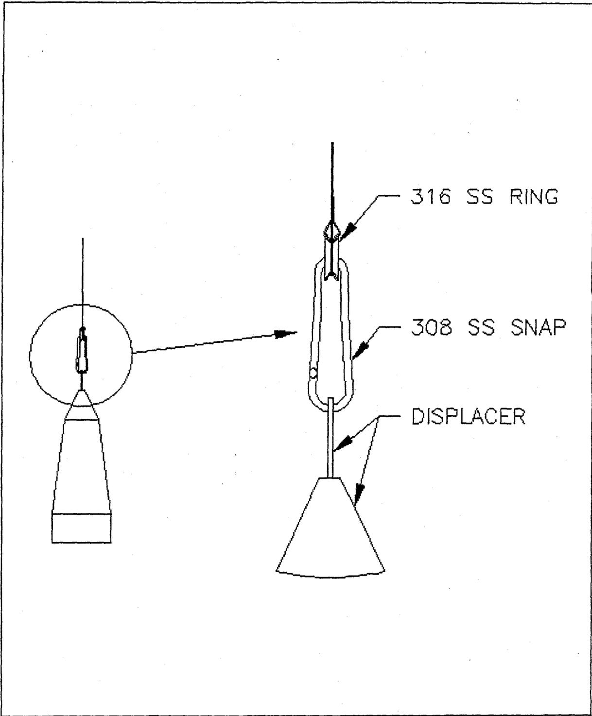
FIGURE 1 - ENRAF gauge 316 ring and displacer assembly
