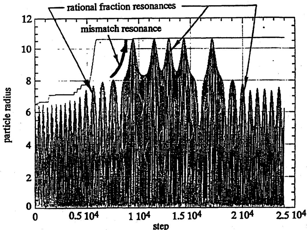
Fig. 8. Mismatched Hamiltonian initial distribution in a continuous, linear focusing channel, with space-charge factor = 0.54 and mismatch = 1.30. Solid line is maximum radius of all particles. Oscillating line is the detailed radius of the particle that achieved the maximum radius during the run, showing that the dynamics involves many rational fraction resonances as well as the main mismatch resonance.
