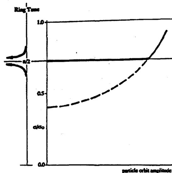
Fig. 9. Tune depression diagram for a system with a very strong resonance.
