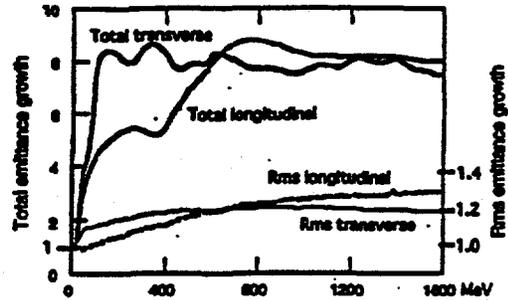
Fig. 1. Beam size and emittance behavior in a 1 GeV proton rf linac, with constant accelerating gradient and  $\sigma_0^{\dagger}$  per unit length.
