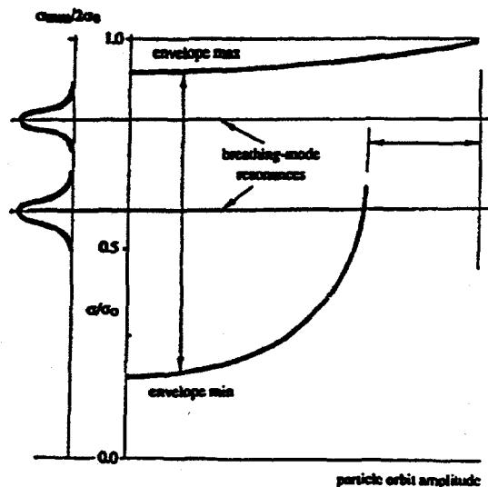
Fig. 7. Tune depression excursion for a radially mismatched beam.
