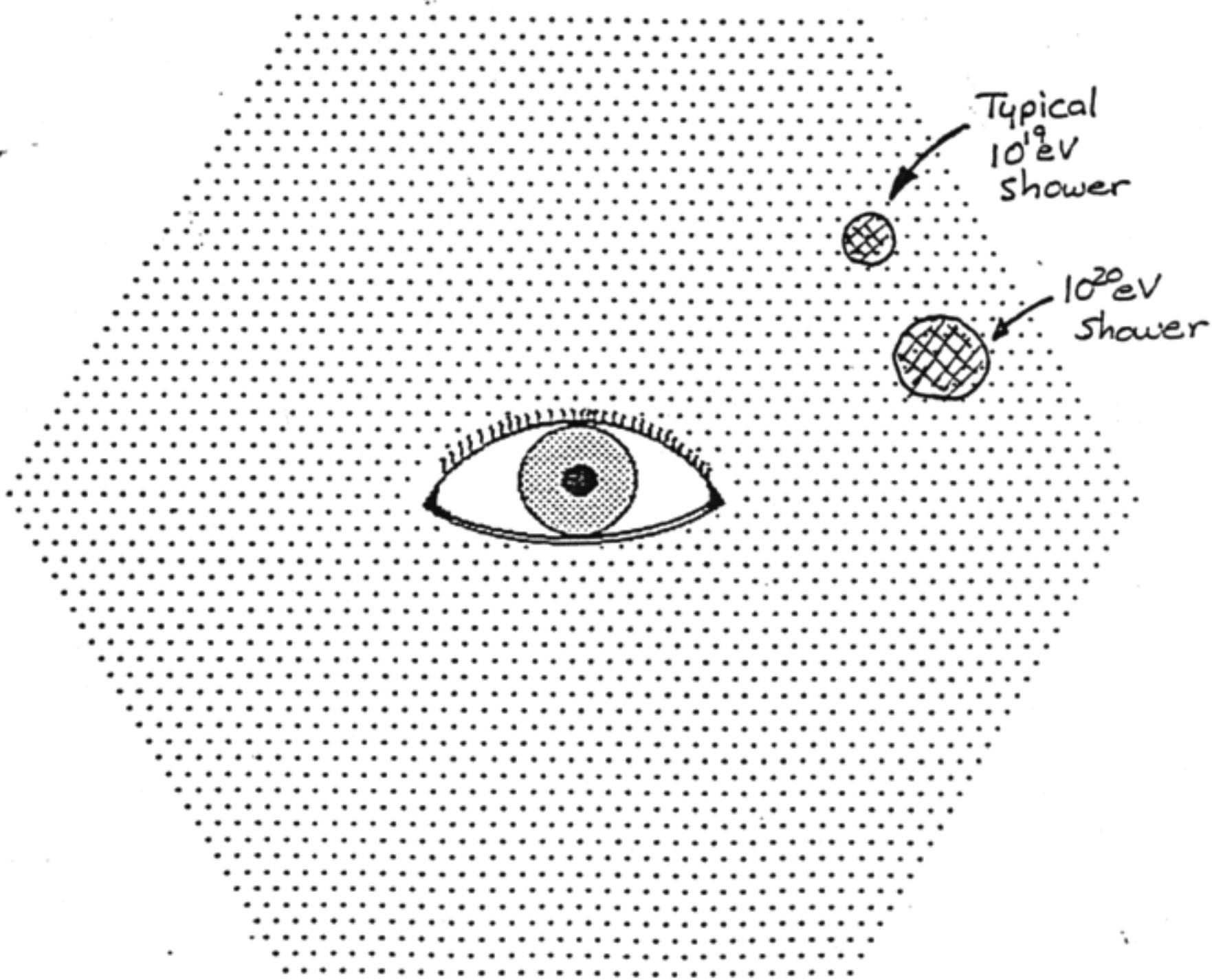
**FIGURE 9.** Cartoon of the ground array with fluorescence "eye" in the center. The circles are the approximate size of  $10^{19}$  and  $10^{20}$  eV showers.
