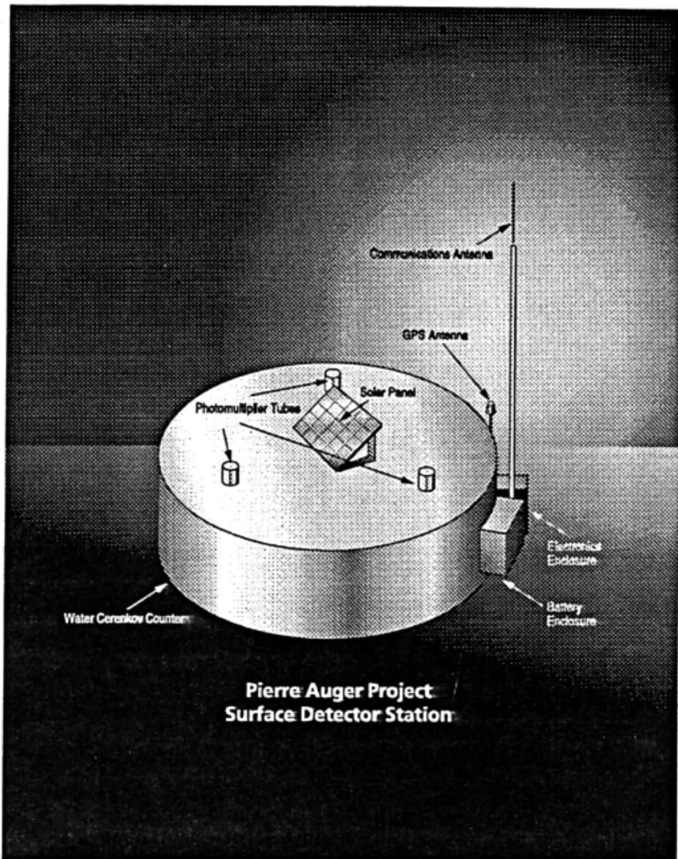
**FIGURE 10.** Conceptual design for the Water Cerenkov detector for use in the surface array.
