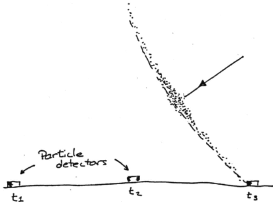
**FIGURE 7.** Illustration of cosmic ray direction measurement using air shower front.
