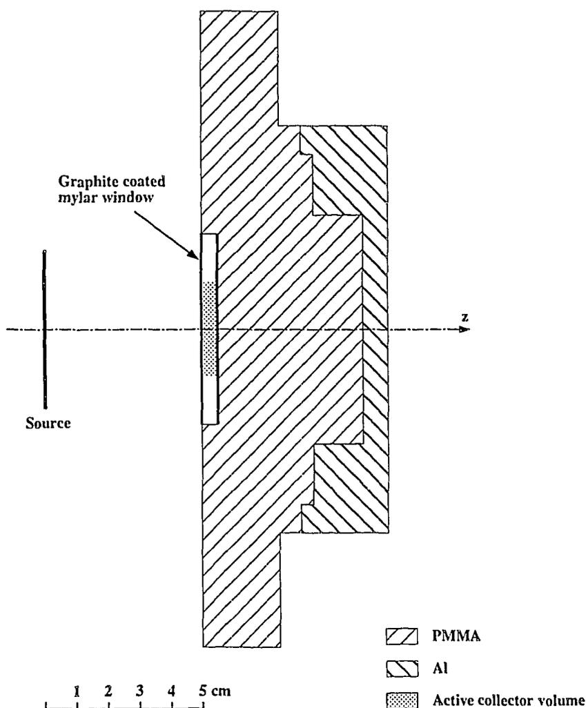
Figure 5. Extrapolation chamber configuration in MC calculations. It is similar to the extrapolation chamber used at NRC, though screws and connectors have been simplified to PMMA in the MC model.
