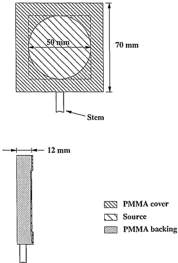
Figure 1. The configuration of the physical source including source holder (backing and cover) of PMMA.
