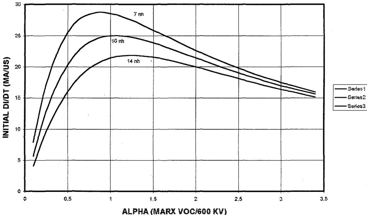
**Figure 7** Variation in di/dt with Bank Voltage.
