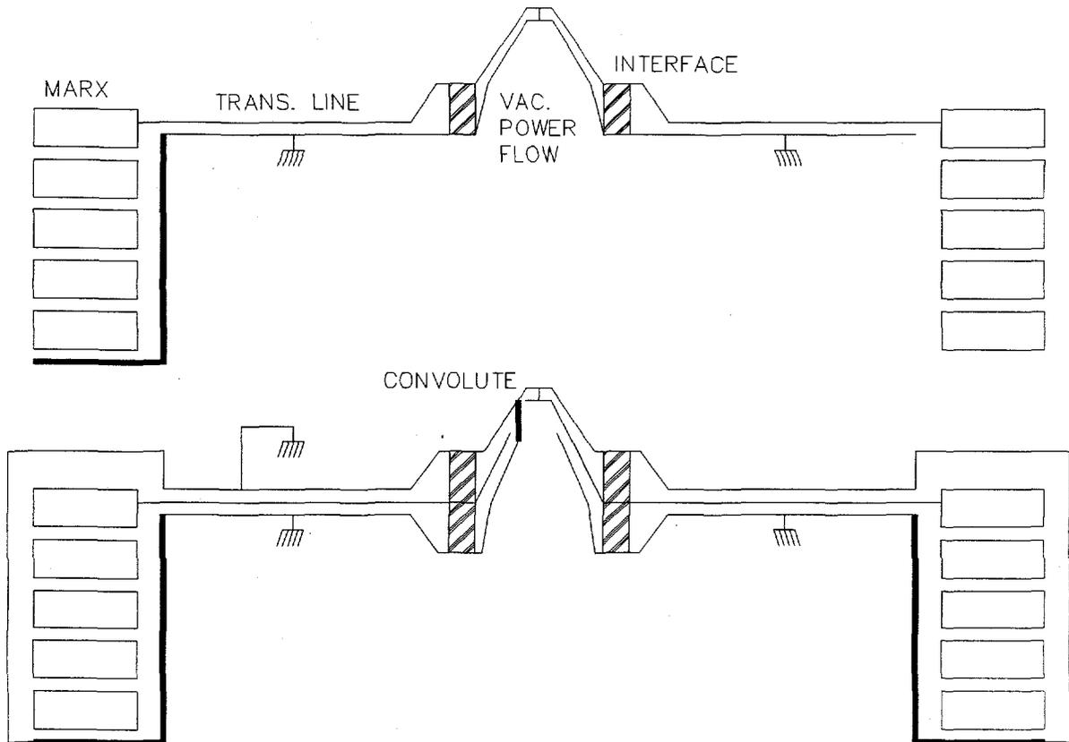
**Figure 8** Simplified sketch of the Atlas bank with a convolute supplied to reduce overall inductance.
