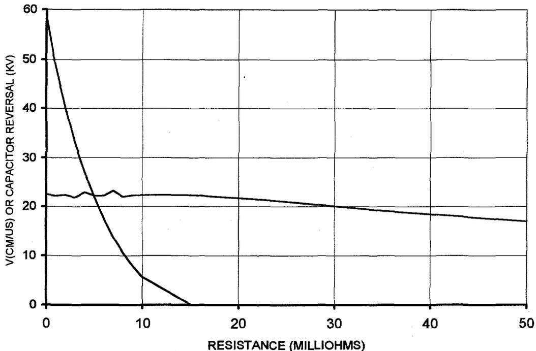
**Figure 2** Implosion velocity as a function of series resistance for the baseline case of 36 mg and 600 kV.
