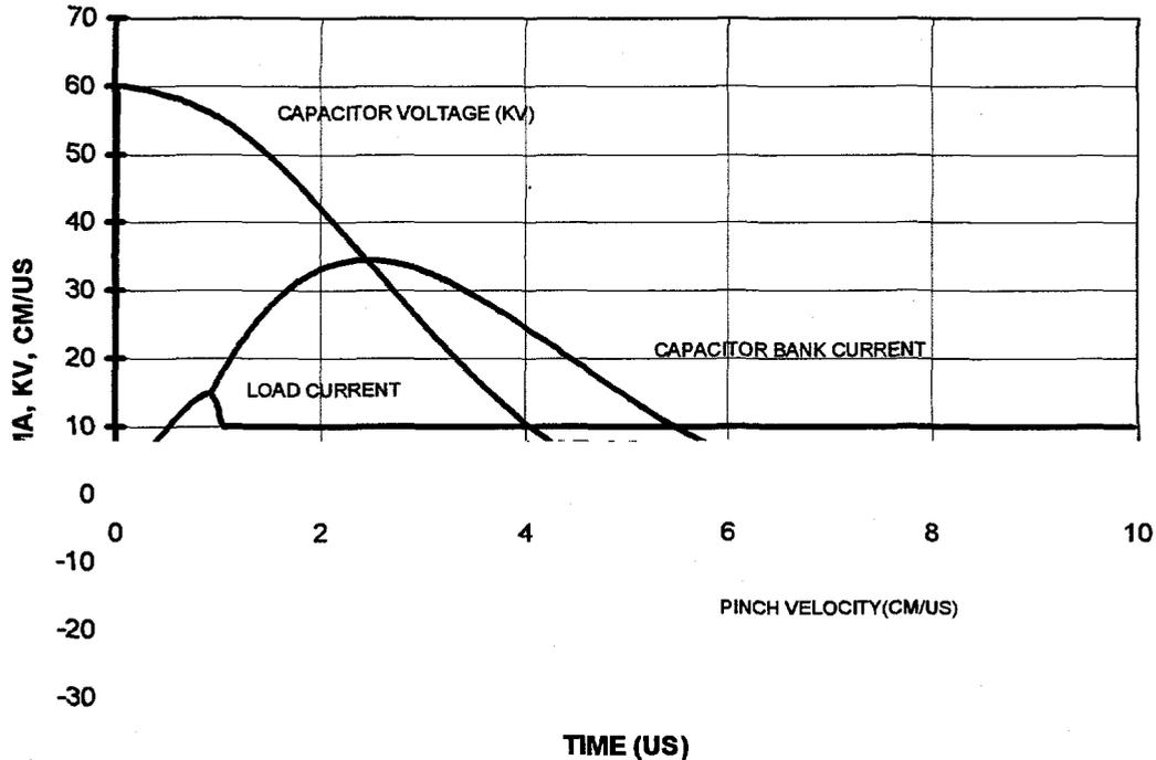
**Figure 4** Typical output traces for 36 mg load, 600 kV charge, and 200 uf bank capacitance.
