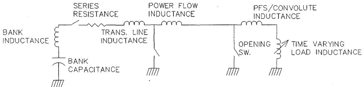
**Figure 1** The circuit simulated is shown above. The Atlas3 code simulates the circuit without the opening switch, and Atlas4 simulates the opening switch.
