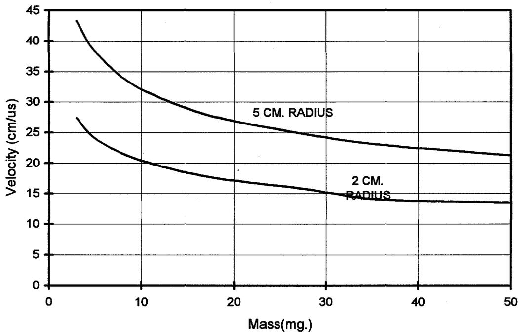
**Figure 5** Implosion velocity dependence on mass and radius for direct drive.
