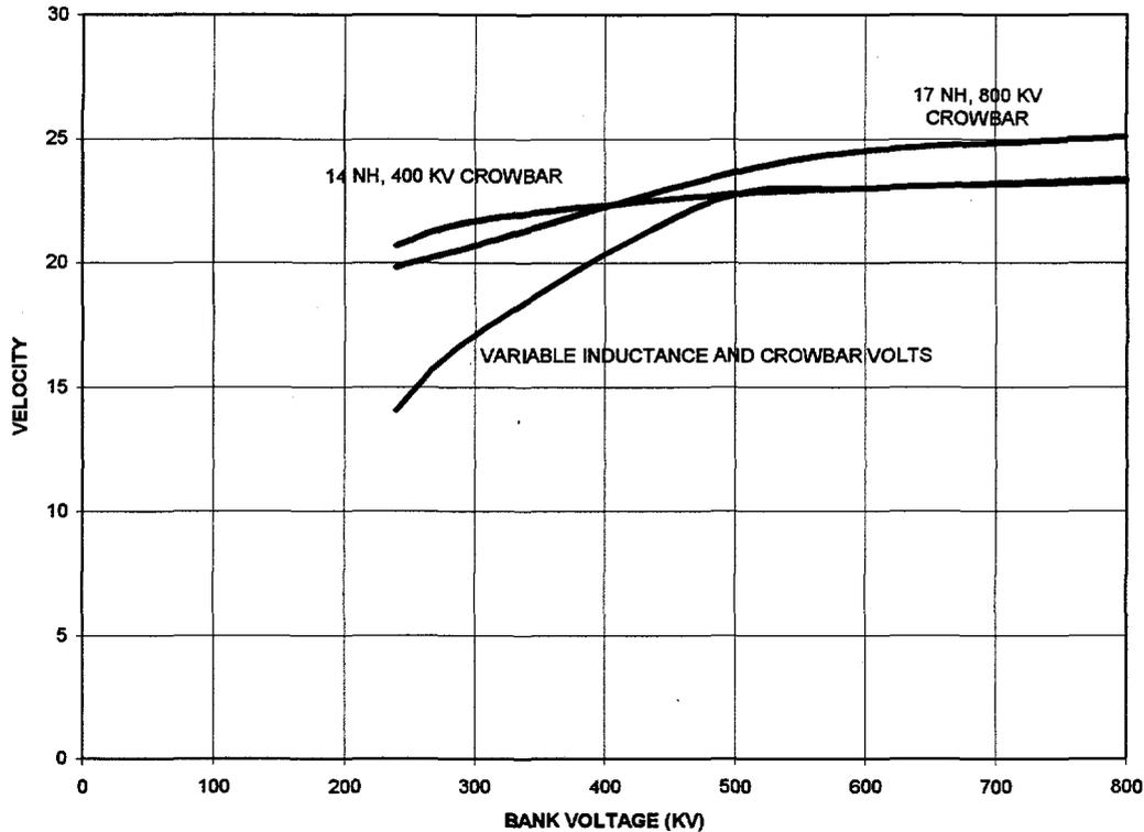
**Figure 6** Direct drive implosion scaling with bank voltage. The crowbar voltage and power flow inductance are varied linearly in the variable case.
