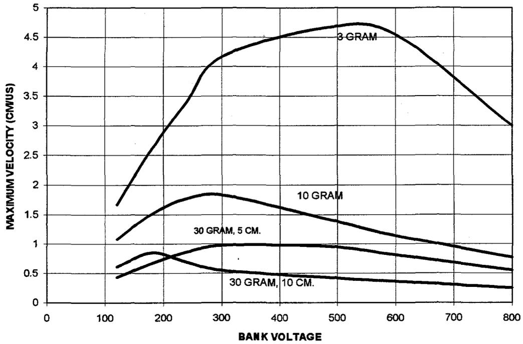
**Figure 3** Heavy liner velocities for 3, 10 and 30 grams with 5 and 10 cm. radii studied for the 30 gram case.
