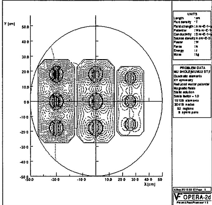
correspondingly high. But for the minimum cost the number of recirculations appears to be of the order of 20 - a relatively high number. In order to avoid a large number of separate magnets, multiple aperture magnets can be designed (see Fig.6).
