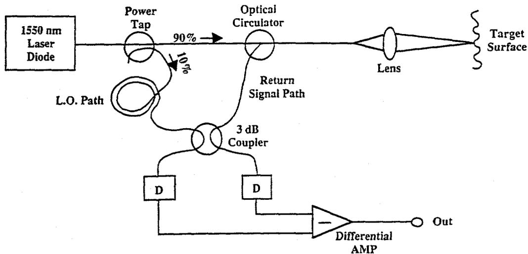
Figure 2-2. Basic Fiber Optic FMCW CLR Configuration
