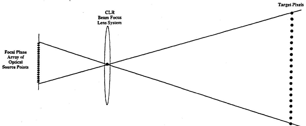
Figure 2-4. Simplified Schematic of Fiber Optic-Based Scanner
