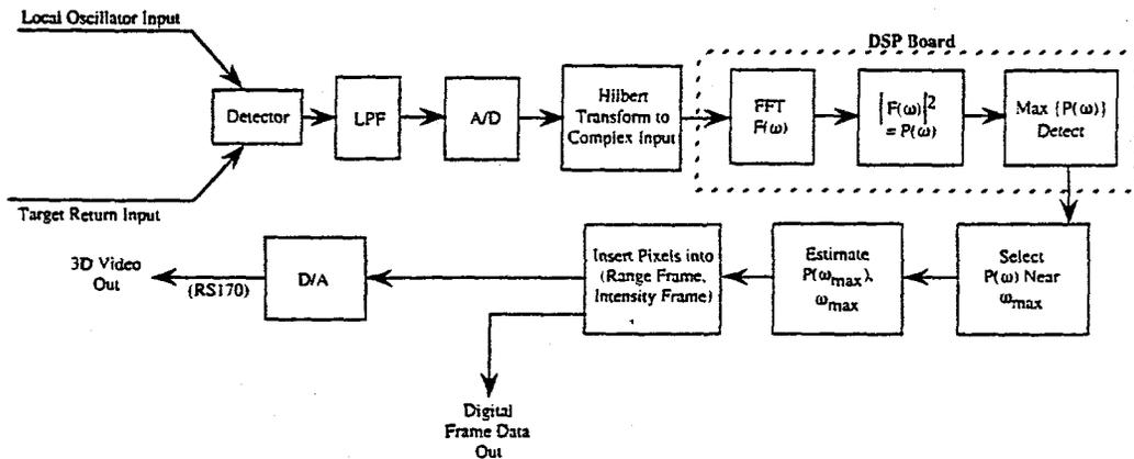
Figure 2-5. CLR 3D Vision Receiver Processor
