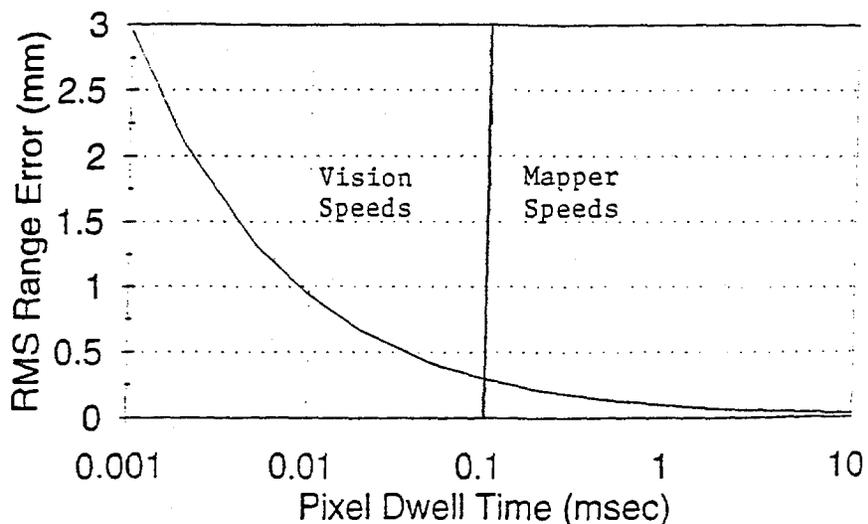
Figure 1-1. Coherent laser radar accuracy vs. pixel dwell time. Laser radar parameters: 50 GHz tuning 1cm aperture, 10mW optical power, 10m range.
