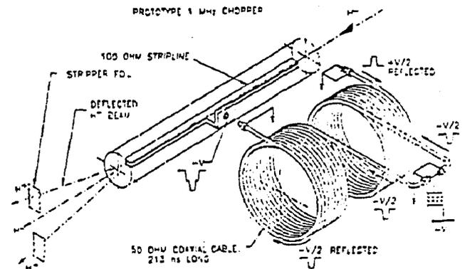
Fig. 4. Schematic diagram of rf beam chopper.
