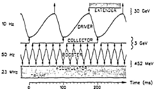
Fig. 1. Energy-time plot showing the progress of the beam through the five rings.
