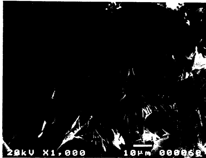
Fig. 2. SEM Photomicrograph of Fracture Surface of Magnesium Phosphate-35 wt.% Ash Final Waste Form.
