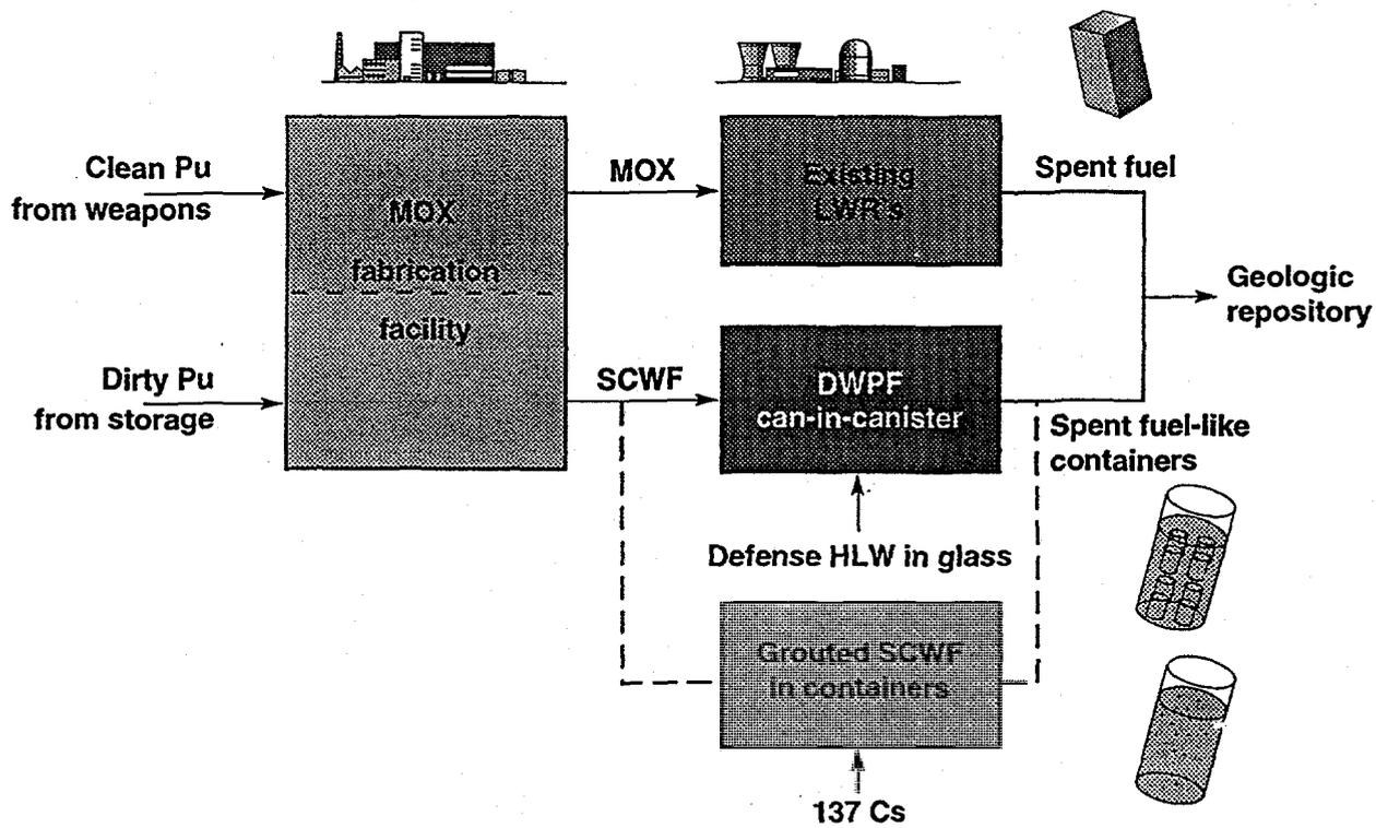
Fig.1 Conceptual disposition of the sintered ceramic waste form (SCWF) using a common MOX fuel fabrication facility
