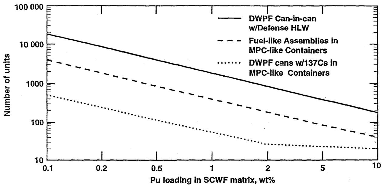
**Fig. 2** Number of DWPF or MPC-like containers required to dispose of 10 t impure Pu vs Pu loading in SCWF matrix
