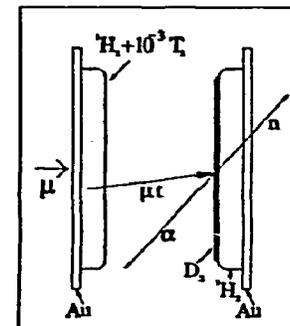
The target is made of two gold foils which are cooled to 3K. The distance between these foils is variable from 18mm to 40mm. A two sided gas diffusion mechanism allows the deposition of different types of hydrogen mixtures on the two foils. After a target deposition, the diffuser is removed. Fig. 2 shows a target configuration. Important features, considered during the design of the target system, were use of tritium and a limit on the number of materials in which a muon can stop.
