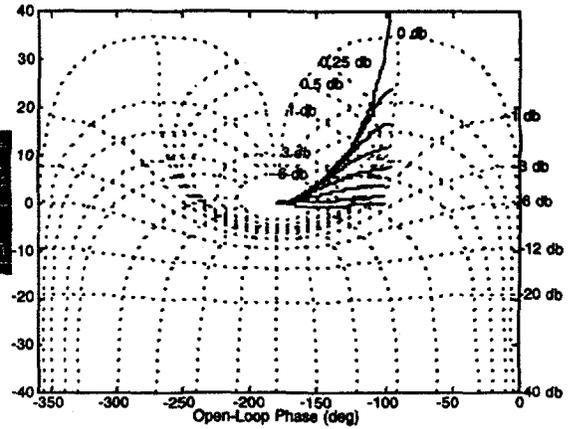
Fig. 8. Nichols plot of the model for the elbow joint of the Schilling Titan II slave manipulator showing the effect of joint nonlinear friction and compliance (Describing function method).
