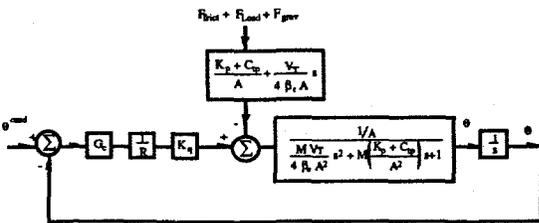
Fig. 6. Block diagram of the joint controller.
