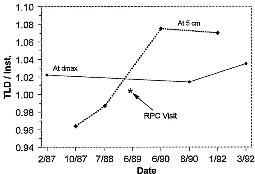
*Figure 1 - Results of six mailed TLDs over a 5-year period on a 6-MV x-ray beam. The results of ion chamber measurements by the RPC on this beam in 1989 are also included. The results appeared to have wide variations until the trend was identified. The institution calibrated the beam either by measurements at  $d_{max}$  or a 5-cm depth in a polystyrene phantom. The disparity between the two is presently under investigation.*
