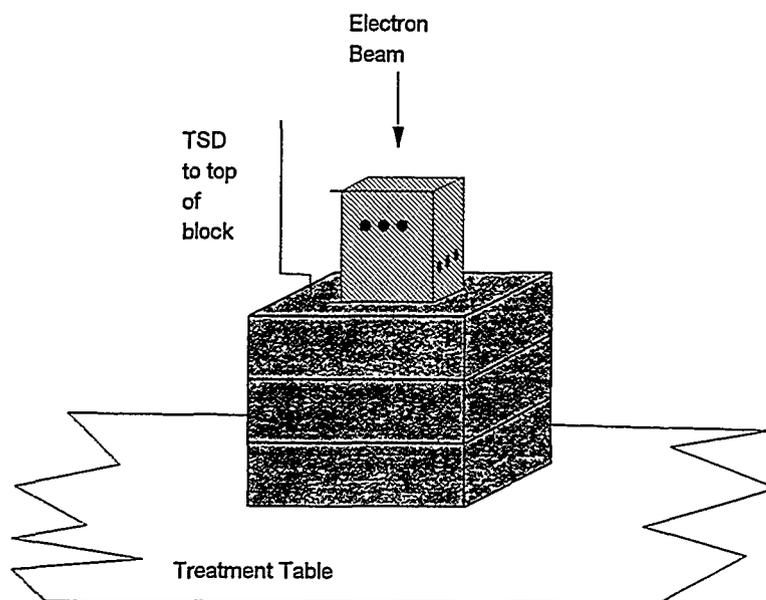
**Figure 3 - Schematic Diagram of the electron irradiation geometry. The block holding the TLDs is shown partially withdraw to demonstrate the location of the two sets of TLDs, one near  $d_{max}$  and one in the fall-off region.**
