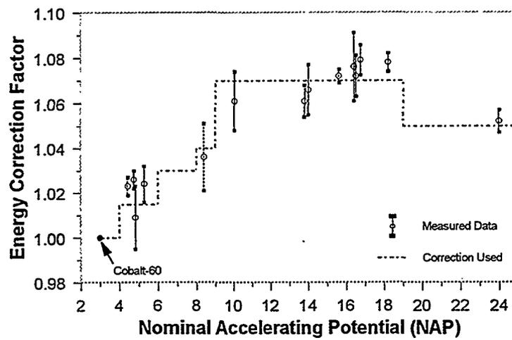
*Figure 5 - Dependence of the TLD system on the photon energy. Various irradiation blocks are used over a range of energies. The correction factor used is specific to the block and is indicated by the dashed line.*
